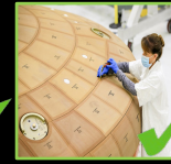
HEAT SHIELD BLOCK INSTALL COMPLETE
