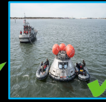
*CREW MODULE UPRIGHT SYSTEM TEST
