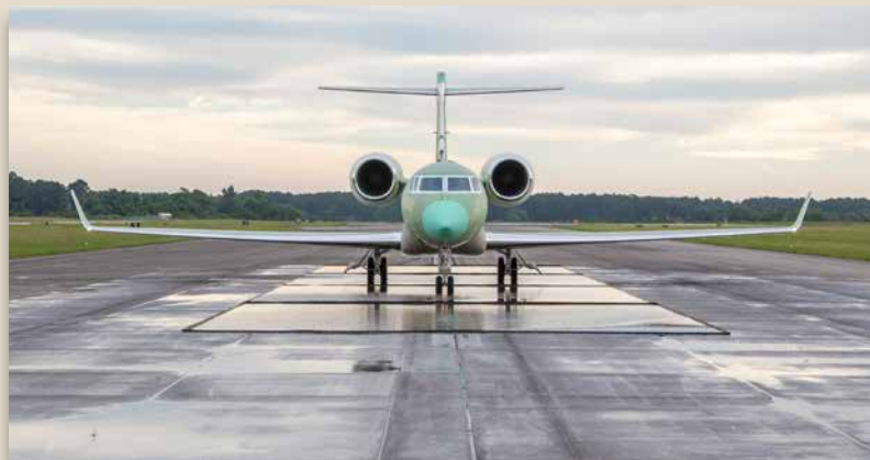
The Gulfstream G500 sits within the water trough on the Wallops airfield.
