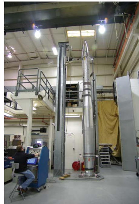
Figure 6.5: Payload Undergoing Bend Test at WFF
