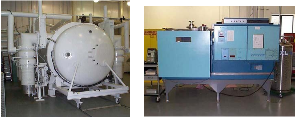
Figure 6.4: PV/T Vacuum Chamber (left) and Tenney Space Simulation System Thermal Vacuum Chamber (right) at WFF
