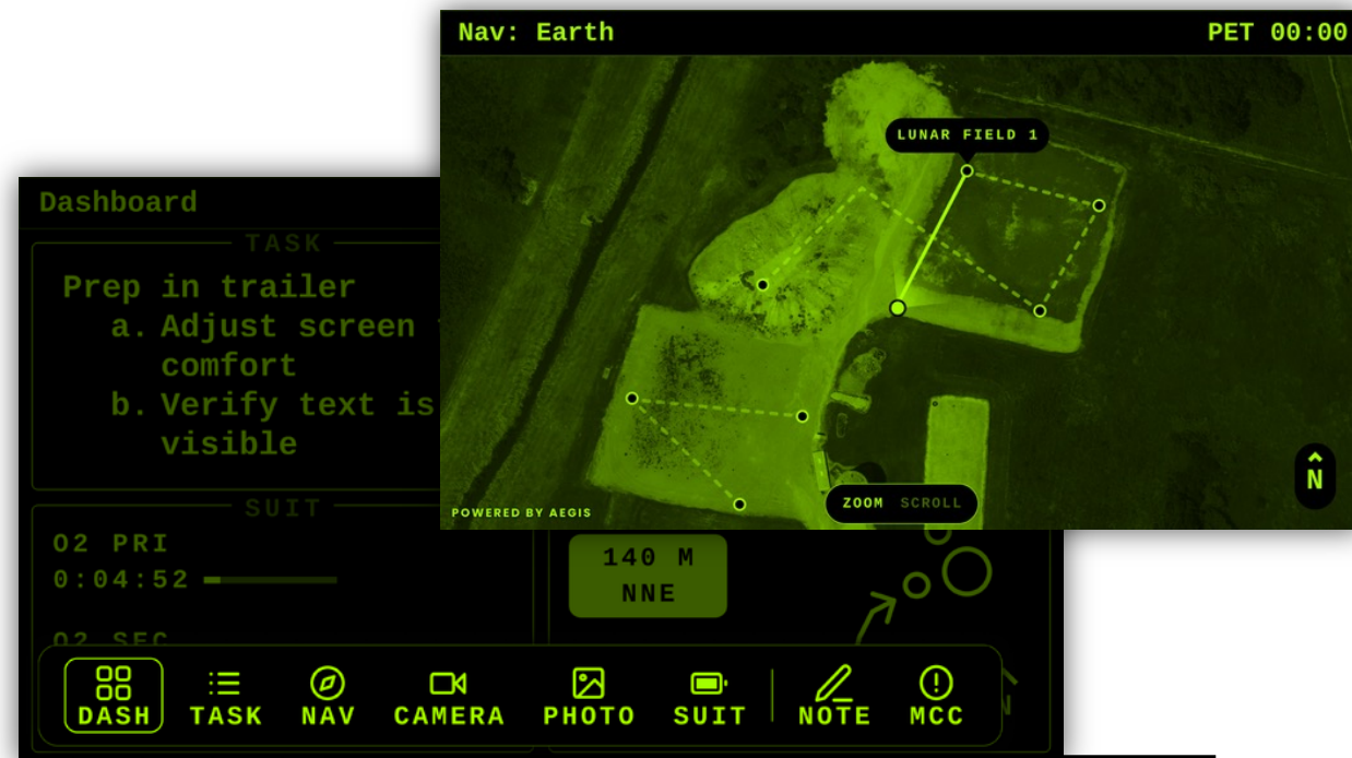
Joint AR Custom Graphics Engine - STARK Rendered User Interface Application: procedures, navigation (2D AEGIS Maps), camera view finder, photos, suit consumables, notes, and MCC messages
