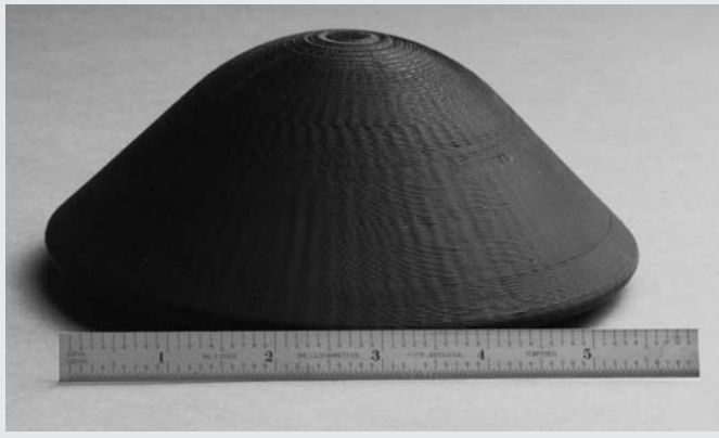
Model of the Reentry Breakup Recorder (spacecraft 'black box') to scale. The addition of the heat shield is expected to bring its size closer to 1 foot (0.3 meters) in diameter.
