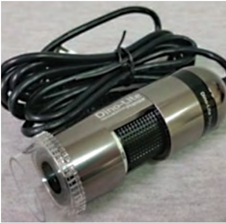
NanoRacks Microscope-3 is an off-the-shelf Universal Serial Bus (USB) microscope. Image courtesy of NanoRacks LLC.
