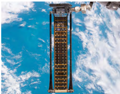
The Roll-Out Solar Array (ROSA) is a new type of solar panel that rolls open in space like a party favor and is more compact than current rigid panel designs.
