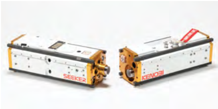
Seeker, an automated extravehicular free-flying inspector CubeSat, and its communication link, Kenobi. The primary objective of the Seeker mission is to demonstrate a path toward an inspection capability for future crewed space missions.
