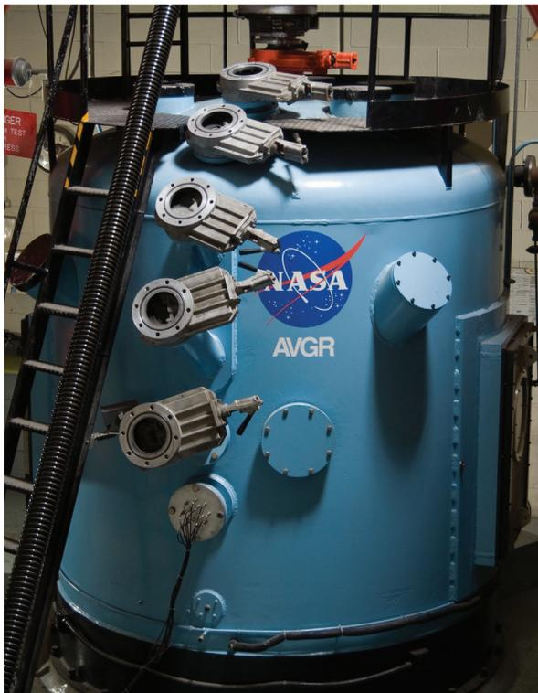
Figure 4.2.2.7. Impact vacuum tank (exterior view)
