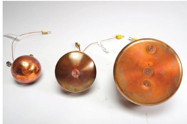
Figure 4.1.5.1. Examples of typical slug-calorimeter probes
