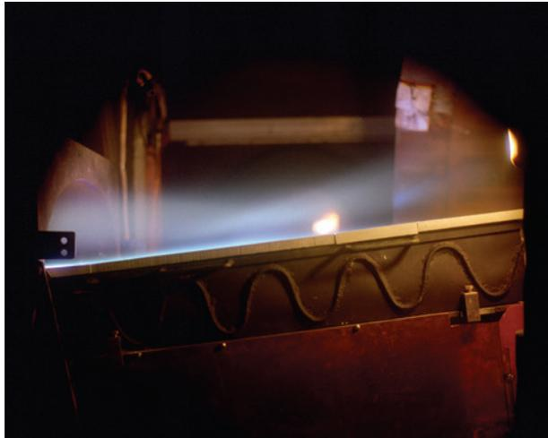
Figure 4.1.0.3. 24x24 in (61x61 cm) panel being tested in the arc jet complex
