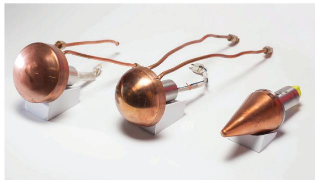
Figure 4.1.5.2. Examples of null-point/coaxial TC calorimeter probes
