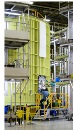
Space Launch System Core Stage-2 (Artemis 2) Intertank is undergoing mechanical assembly at NASA's Michoud Assembly Facility.
