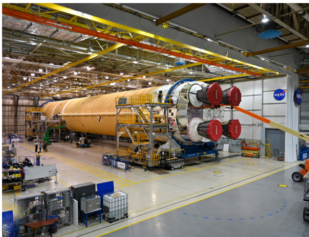
Assembled at MAF, the core stage is complete with all four RS-25 engines, for NASA's Space Launch System rocket.
