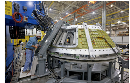
Artemis 3 Orion Pressure Vessel Welding.
