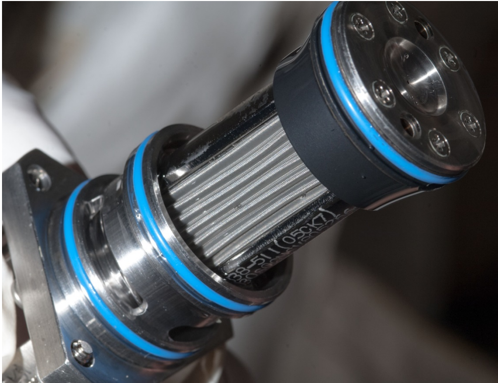
Figure 3-26. Item 141 Gas Trap from EMU 3011 Post-Anomaly
