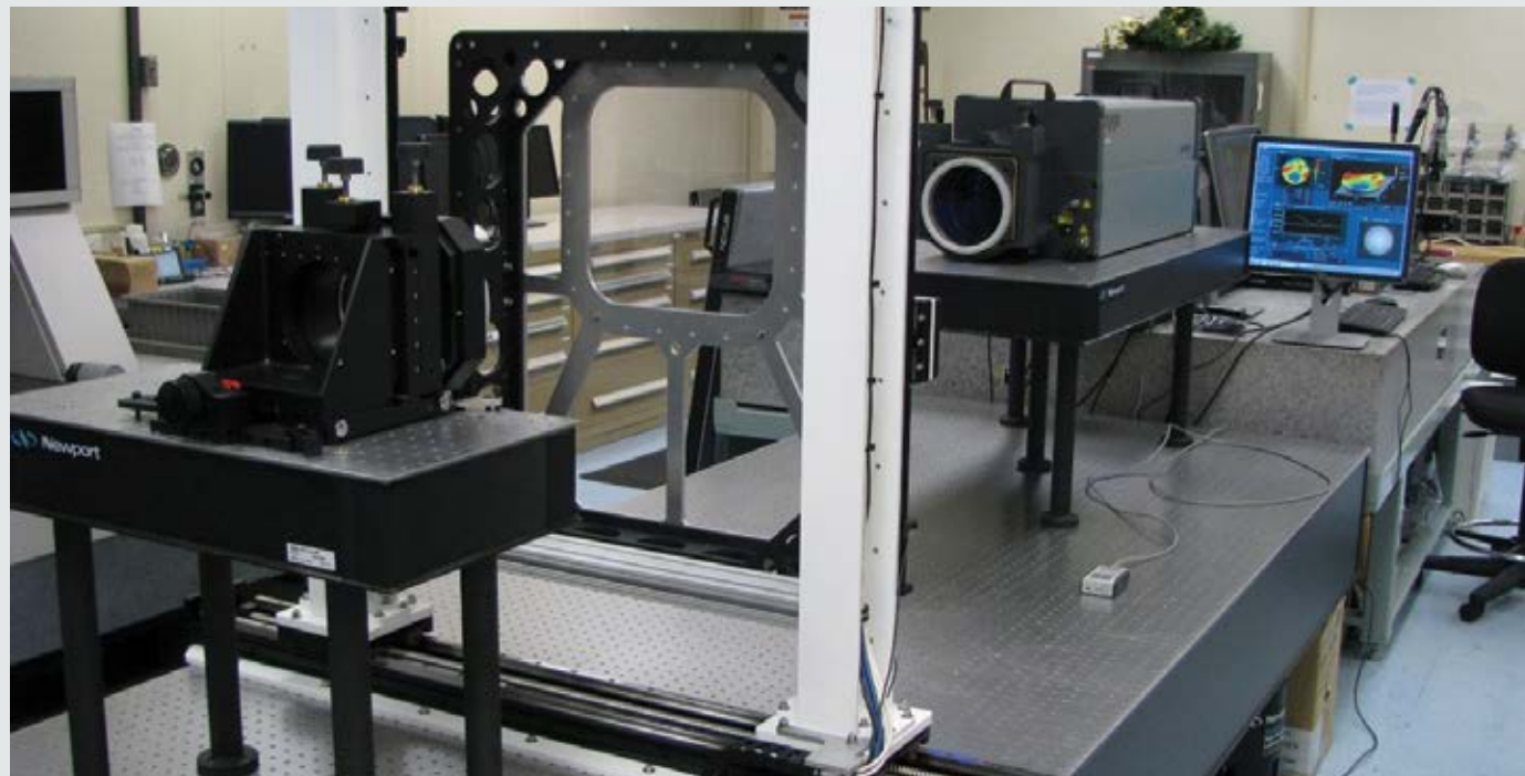
The wavefront measurement system is composed of a 6-inch aperture phase shifting interferometer on a vibration isolated optical table with a 2-D scanning system. This allows the optical path length to be measured across large spacecraft windows as well as individual panes.
