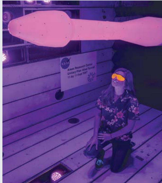
Unsteady pressure sensitive paint applied to generic launch vehicle model in the 11- by 11-foot Transonic Wind Tunnel at ARC.
