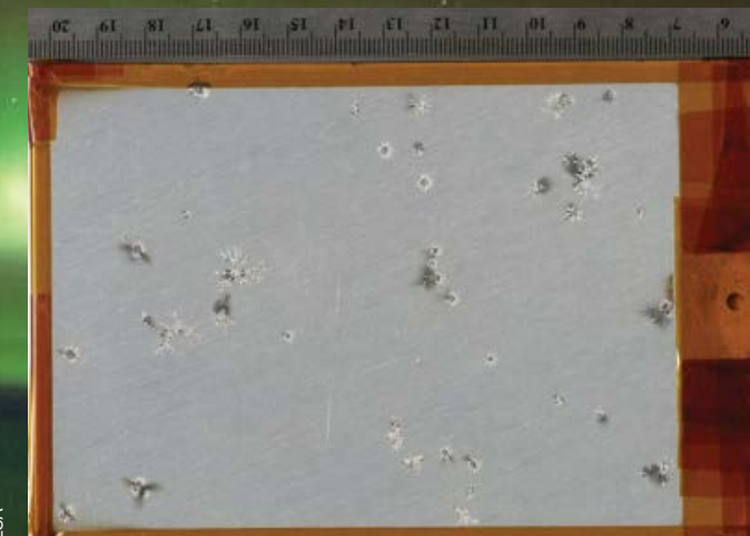
Arc damage in laboratory tests of the chromic acid anodized thermal control coating covering ISS orbital debris shields.
