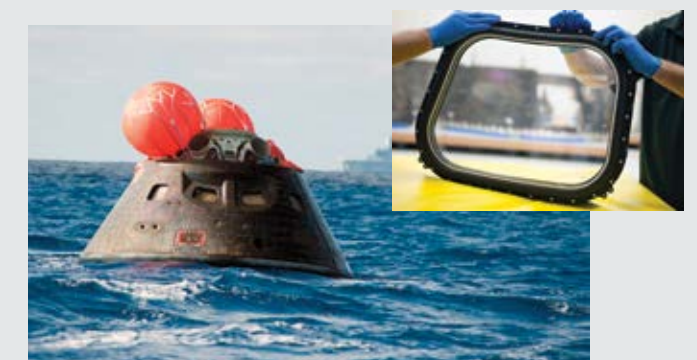
Wavefront measurements were used to characterize Orion CM window flatness.
