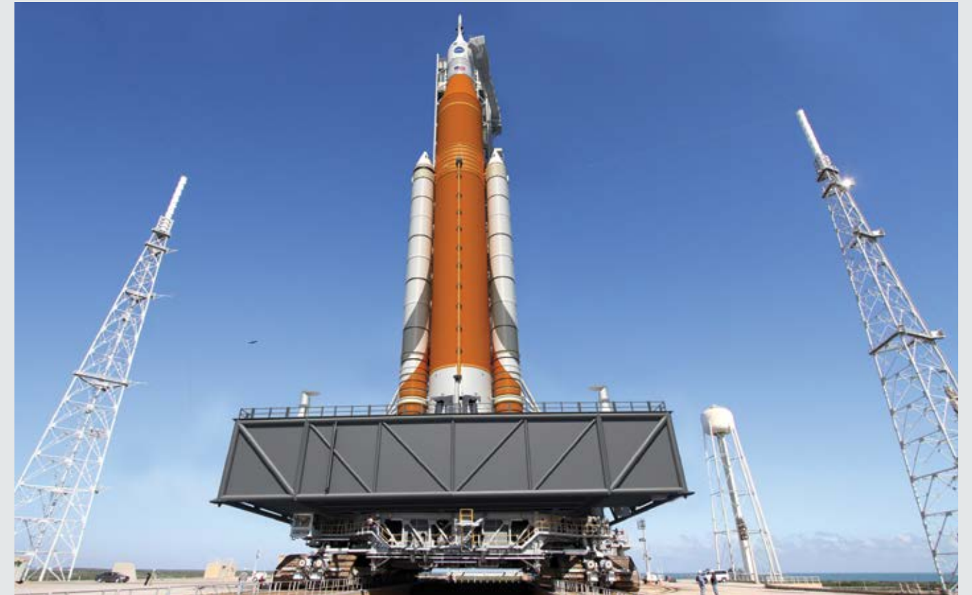
Artist illustration of NASA's SLS launch vehicle and Orion spacecraft on the mobile launcher at Launch Pad 39B at KSC.
