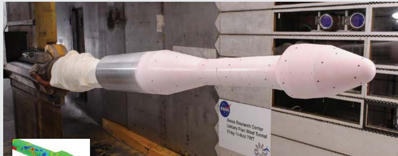
Generic launch vehicle of Coe and Nute covered with pressure sensitive paint and pressure taps.
