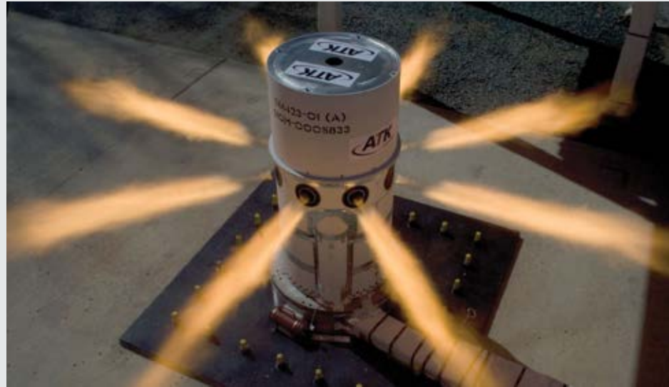
Ground test of a full-scale ACM for the LAS (left). ACM seen operating during the Pad Abort-1 flight test.
