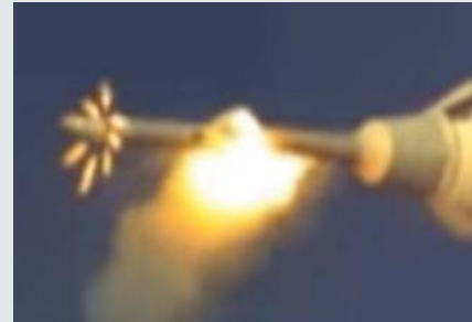
Ground test of a full-scale ACM for the LAS (left). ACM seen operating during the Pad Abort-1 flight test.
