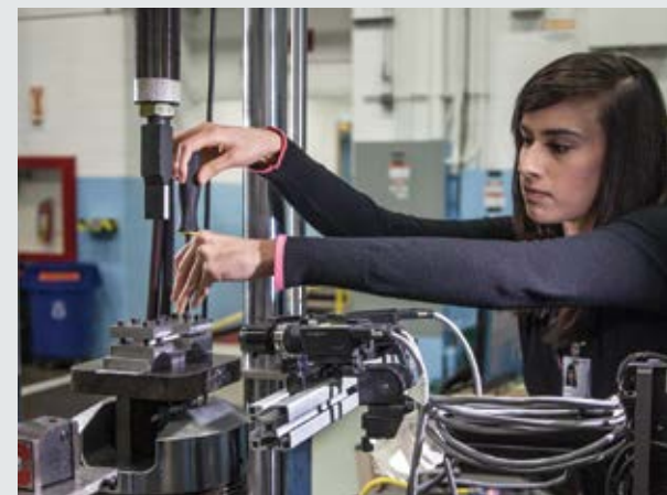
Graduate student Ilse Alcantara and NESC Associate Principal Engineer Jon Haas inspect the pre-test instrumentation set-up of a frangible joint at White Sands Test Facility.
