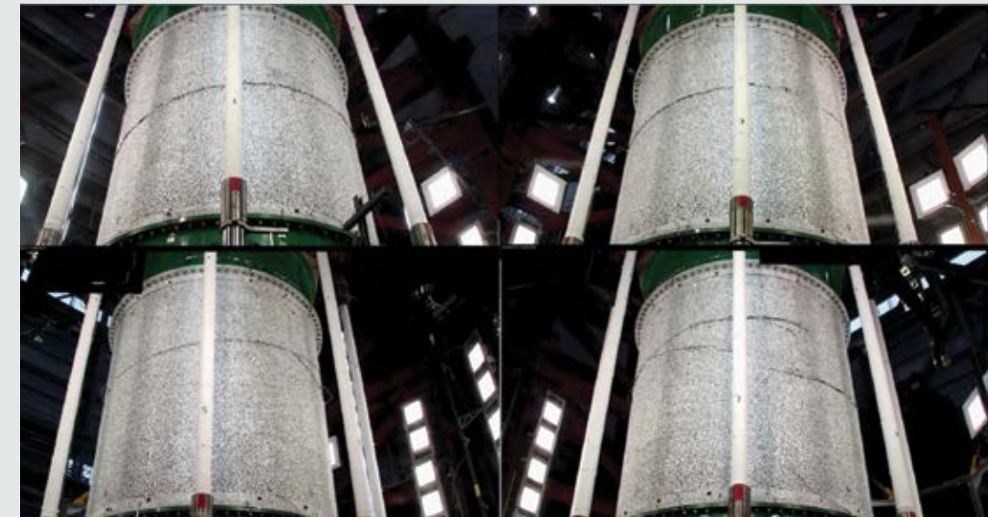
Sector views of failed composite shell.
