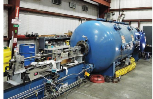
Portion of hypervelocity gun at WSTF
