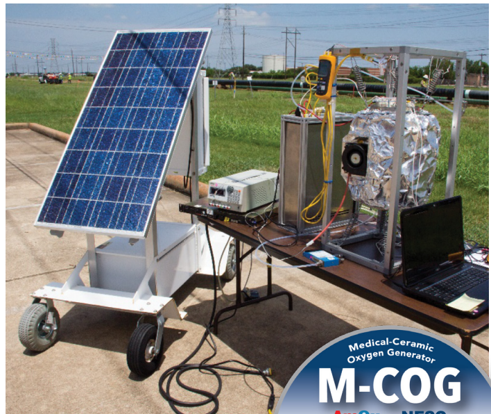
Top: Fully instrumented ceramic oxygen generator prototype; Bottom: Demonstration of a solar powered oxygen generator photographed at JSC in 2012
