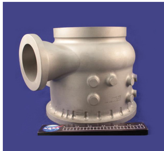
Liquid rocket engine turbopump housing produced using additive manufacturing
