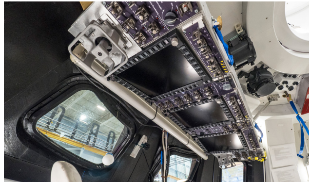
Complex software and hardware will control the Orion crew module. Shown is the Medium Fidelity Mockup at JSC.
