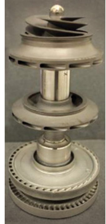
AM parts that make up the rotating assembly of the AM demonstrator engine produced by MSFC
