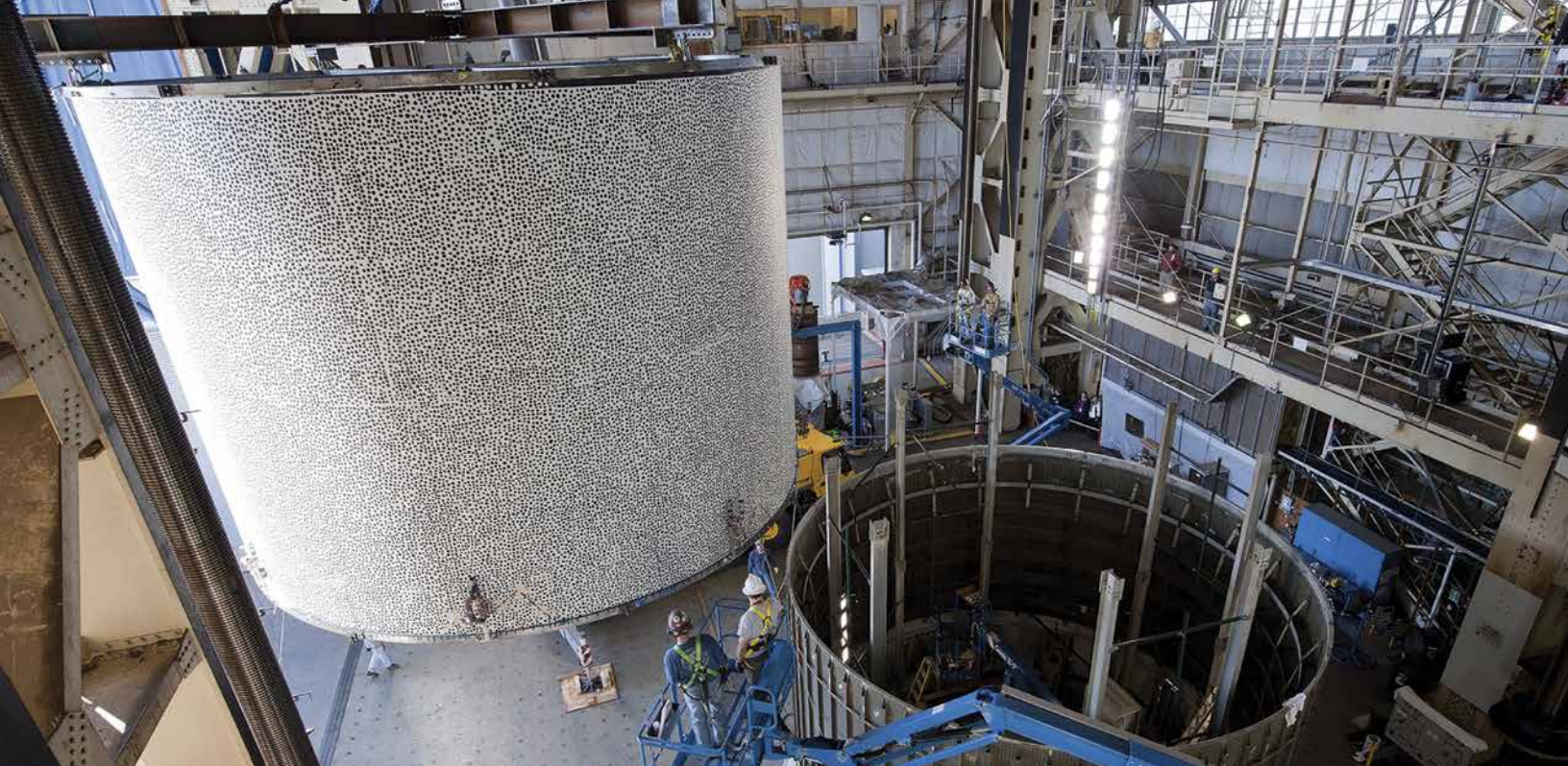
Section of space shuttle external tank covered in photogrammetry targets being mounted in shell buckling test fixture at MSFC.
