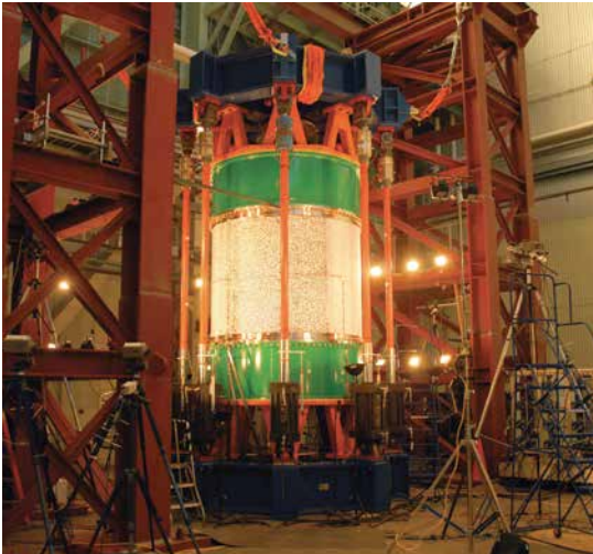
Ares V-style shell undergoing testing at MSFC in 2009.
