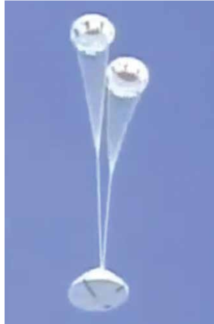
Parachute test vehicle with reefed dual drogues.
