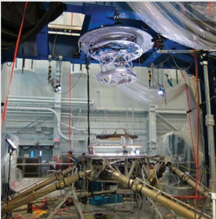
Engineering model of the LIDS being tested in the JSC 6 degrees-of-freedom test stand.
