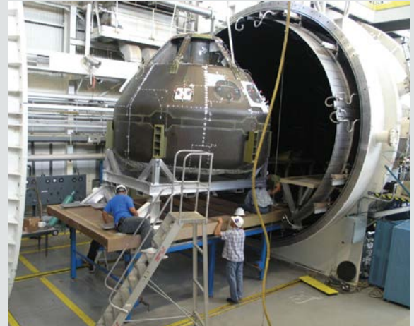
The composite crew module full-scale pressure vessel test article being readied for a vacuum test at MSFC.
