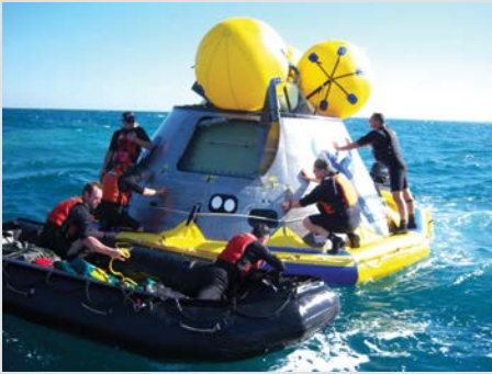
Orion MPCV recovery test article being stabilized during initial testing conducted in 2009.
