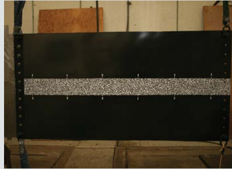
Suspended pathfinder solid laminate composite panel (3 by 6 foot) with photogrammetry speckle pattern and accelerometer attach points.
