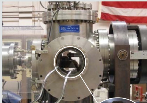
(Above) Vacuum Roller Traction Contract Rig used to characterize vacuum wear marks and debris.
