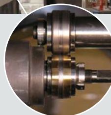
(Above) Vacuum Roller Traction Contract Rig used to characterize vacuum wear marks and debris.
