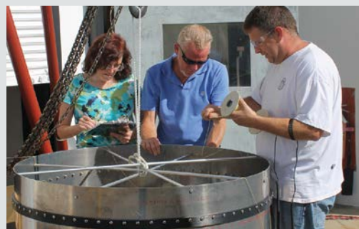
(From left) Maureen Dutton, Rick Dean, Nick Kidd of the JSC Energy Systems Test Branch examine a simulated docking mechanism jettison system tunnel section separation test firing setup.
