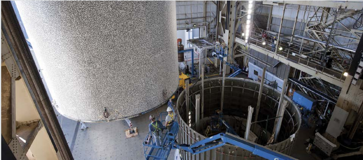
A section of space shuttle external tank covered in photogrammetry targets being mounted in the shell buckling test fixture at MSFC.
