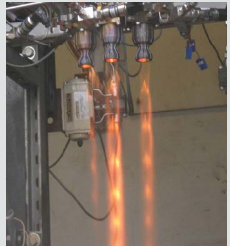
Testing of low-cost engines for nano-launcher upper stage.
