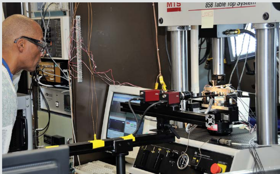
Stewart Walker of the LaRC Advanced Materials and Processing Branch is shown conducting a 3-point strength test on a ceramic C/C-SiC composition material. The specimen is highly instrumented to understand performance.
