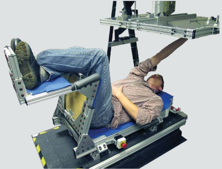
Vibration chair occupant in the ARC Human Vibration Laboratory responding via touch-screen input. Eye and head movement are recorded.
