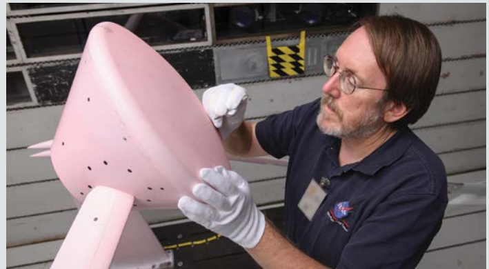
Dr. James Ross prepares a model of the Orion crew module, coated with pressure sensitive paint, in the ARC Unitary Plan Wind Tunnel.
