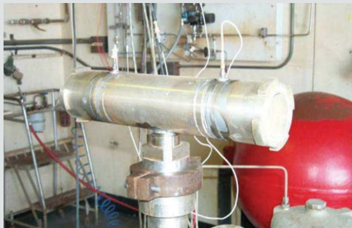
T-burner test rig used for obtaining combustion response data.
