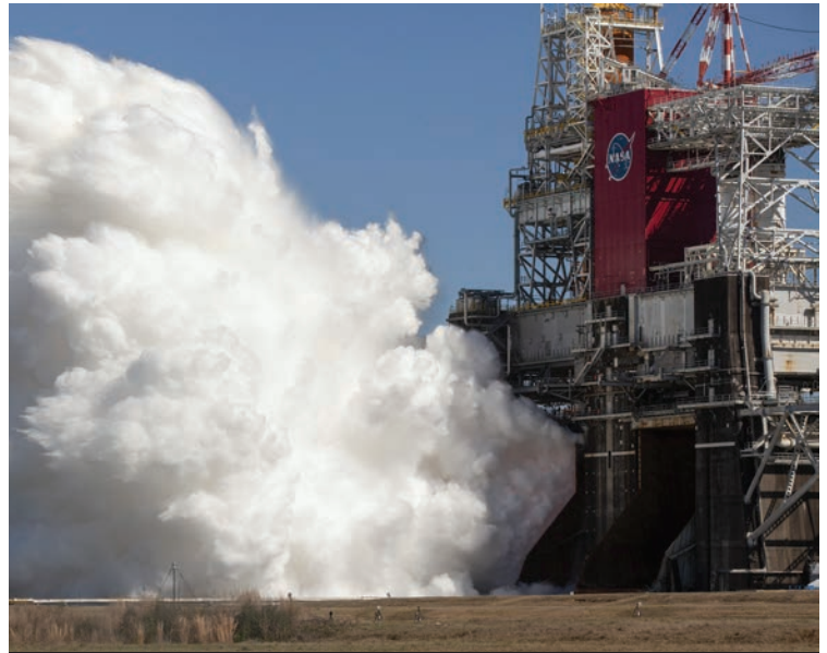
The SLS Artemis I core stage completed a successful, full-duration hot fire at Stennis Space Center March 18.
