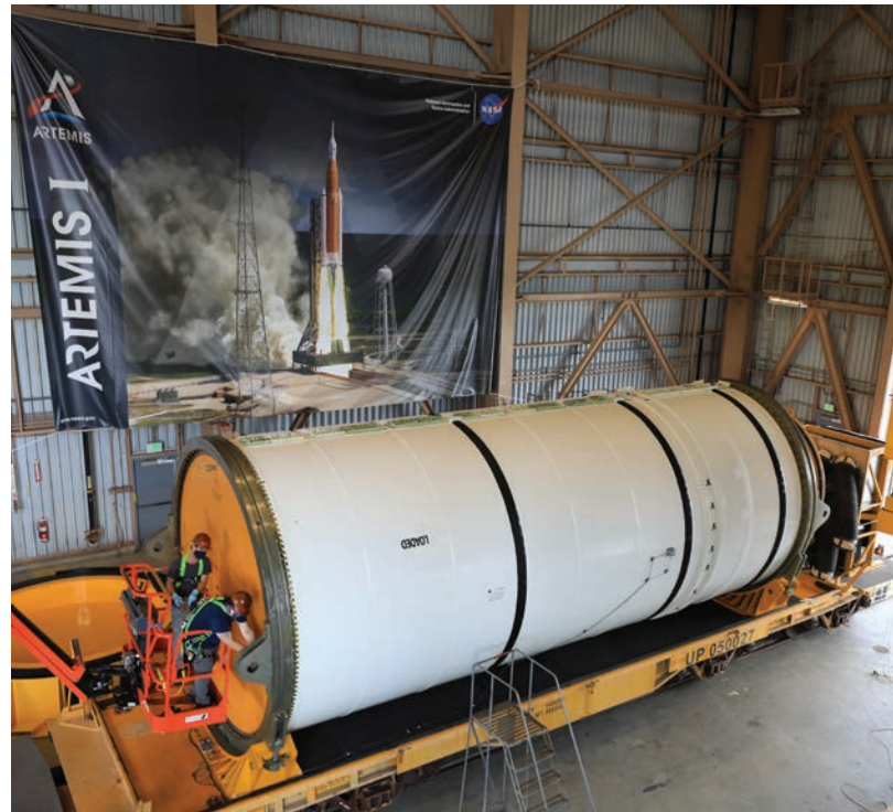
Exploration Ground Systems teams process an SLS solid rocket booster motor segment in preparation for stacking at Kennedy Space Center for the Artemis I mission.
