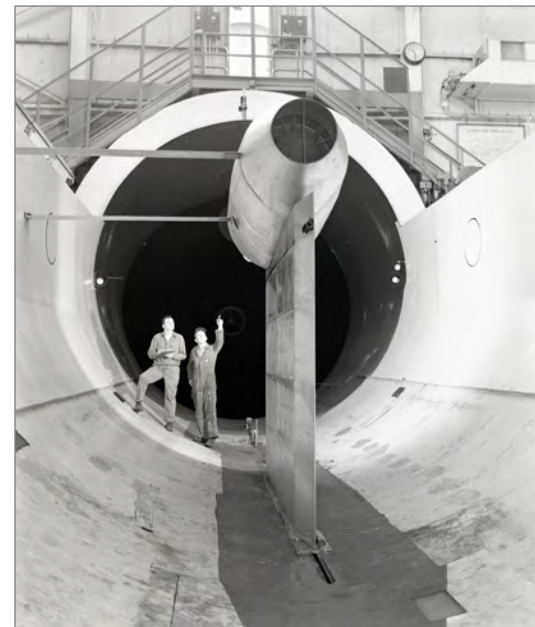
↑ A Pratt & Whitney J57 engine mounted in the AWT in early 1957. The J57, the first U.S. jet engine to exceed 10,000 pounds of thrust, was used in a host of military aircraft including the B-52 Stratofortress, F-100 Super Sabre, and U-2 spy plane. (Photo credit: NACA)
