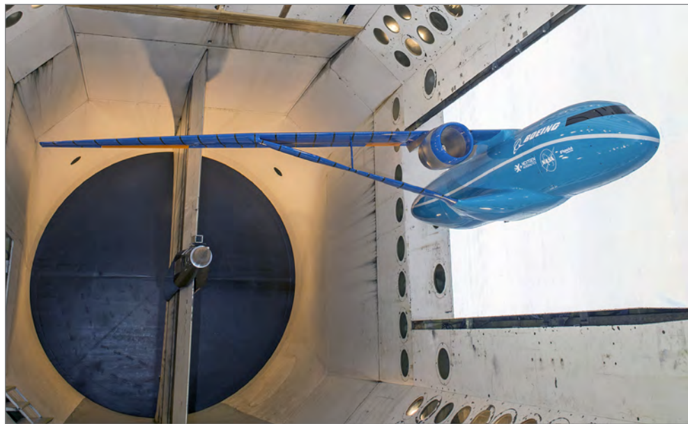
↑ Boeing's 13-foot semi-span Subsonic Ultra Green Aircraft Research (SUGAR) model underwent testing at Langley Research Center's Transonic Dynamics Tunnel in December 2013. (Photo credit: NASA/Langley Research Center/Sandie Gibbs)
