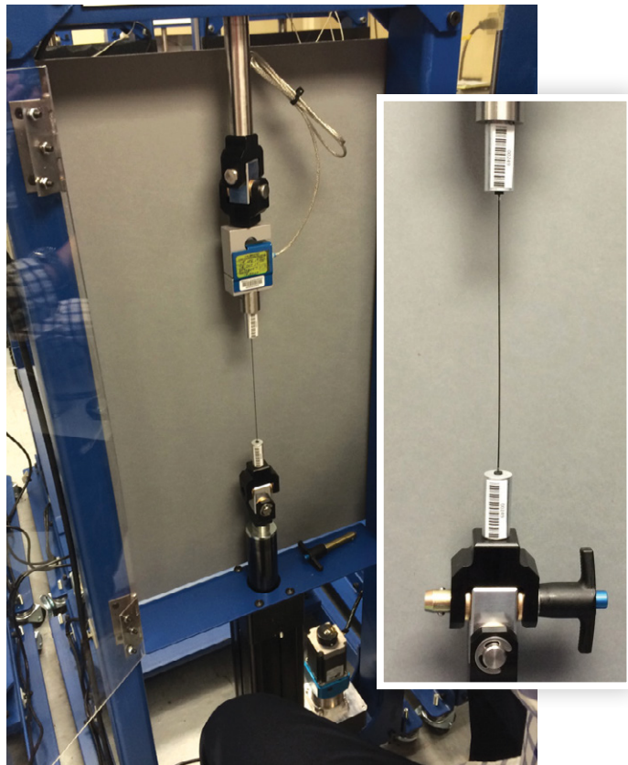
COPVs experience an effect known as stress rupture, where the fibers experience degradation as a function of time, potentially resulting in a sudden overwrap failure and likely catastrophic pressure vessel failure. Shown is stress rupture testing of a carbon fiber strand at room temperature.
