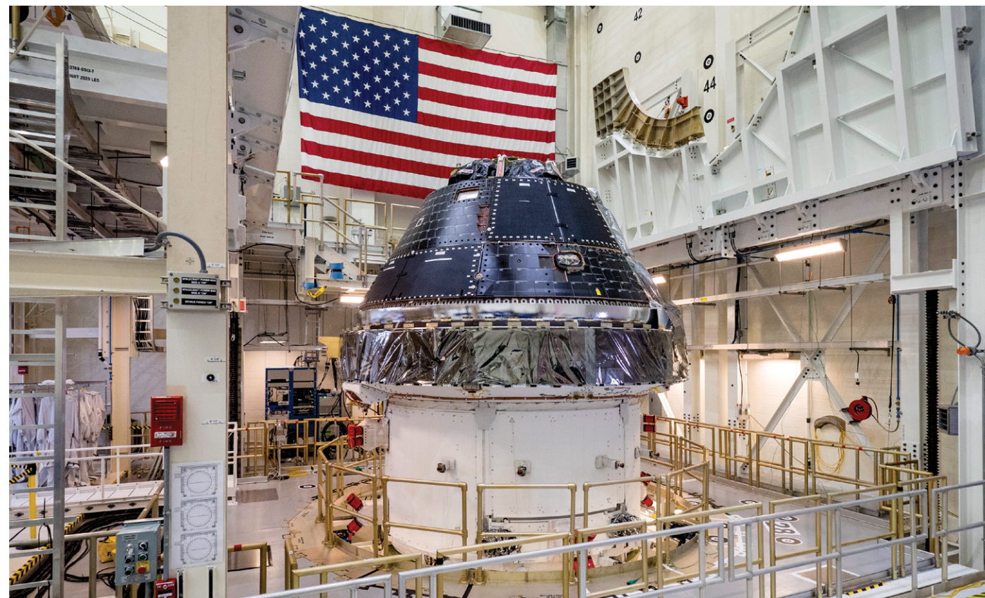
Orion MPCV integration with the European Service Module for the Artemis I mission.
