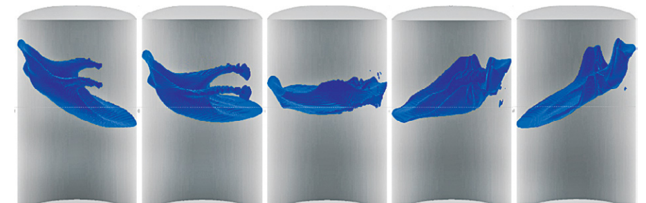
Simulation of slosh in a cylindrical tank.
