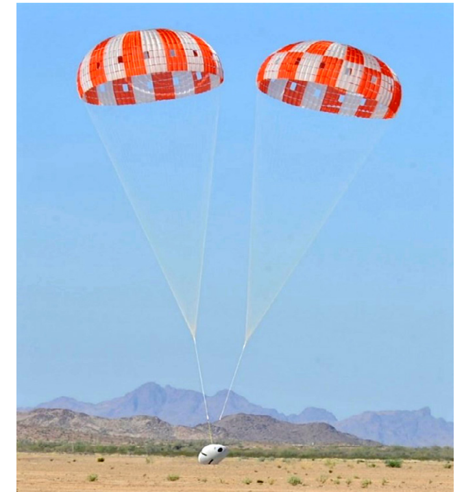
Drop test using only two of three CPAS main parachutes.
