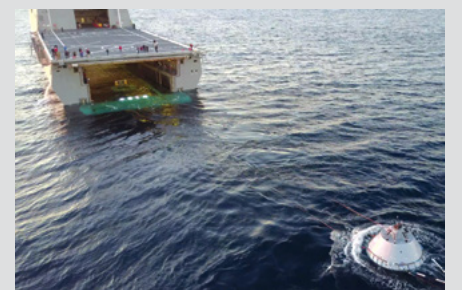
Aerial view of the USS Anchorage as the CM mock-up is recovered into the well deck during URT-7. The image was extracted from video recorded by Jamie Peer of NASA.
