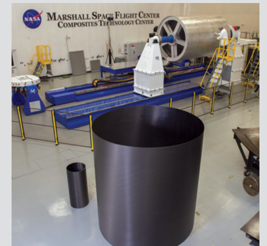
Fabricated composite shells in the MSFC Composites Technology Center
