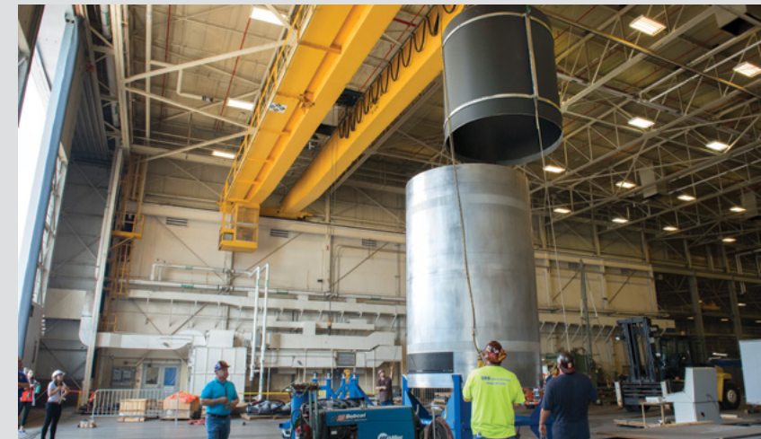
Removal of 8-ft-diameter composite cylindrical test article from fabrication tool at MSFC
