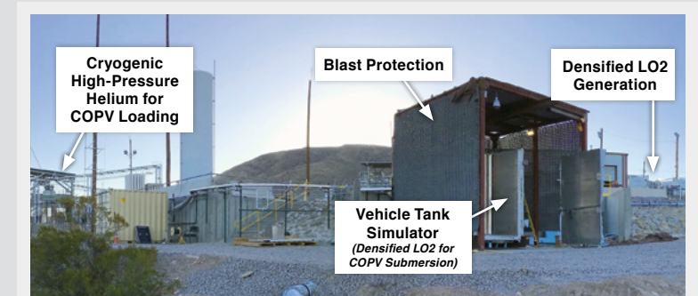
FIGURE 2: COPV flight-like ground test system at WSTF
