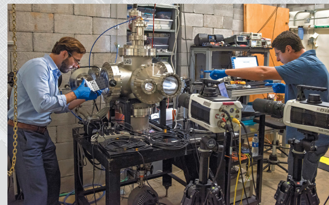
TOP: Dr. Timothy Stephenson (left) and Mr. Stephen Lebar are working on a vacuum bell jar at GSFC where they are collecting particles emitted from electric arcs for analysis in support of the "hot" mate/demate of remote power control modules on the ISS.
