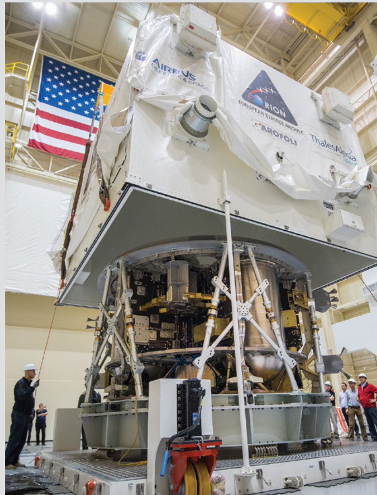
European Service Module being prepared for testing in NASA's Plum Brook Facility
