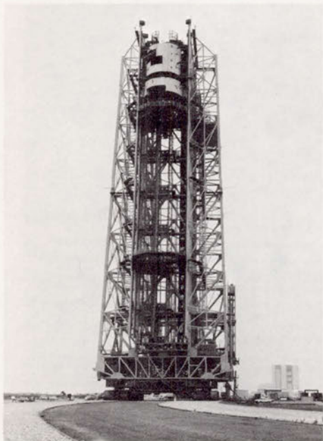
Fig. 116. The crawler carrying the service structure to the pad, 21 October 1966. The assembly building is in the background, right.
