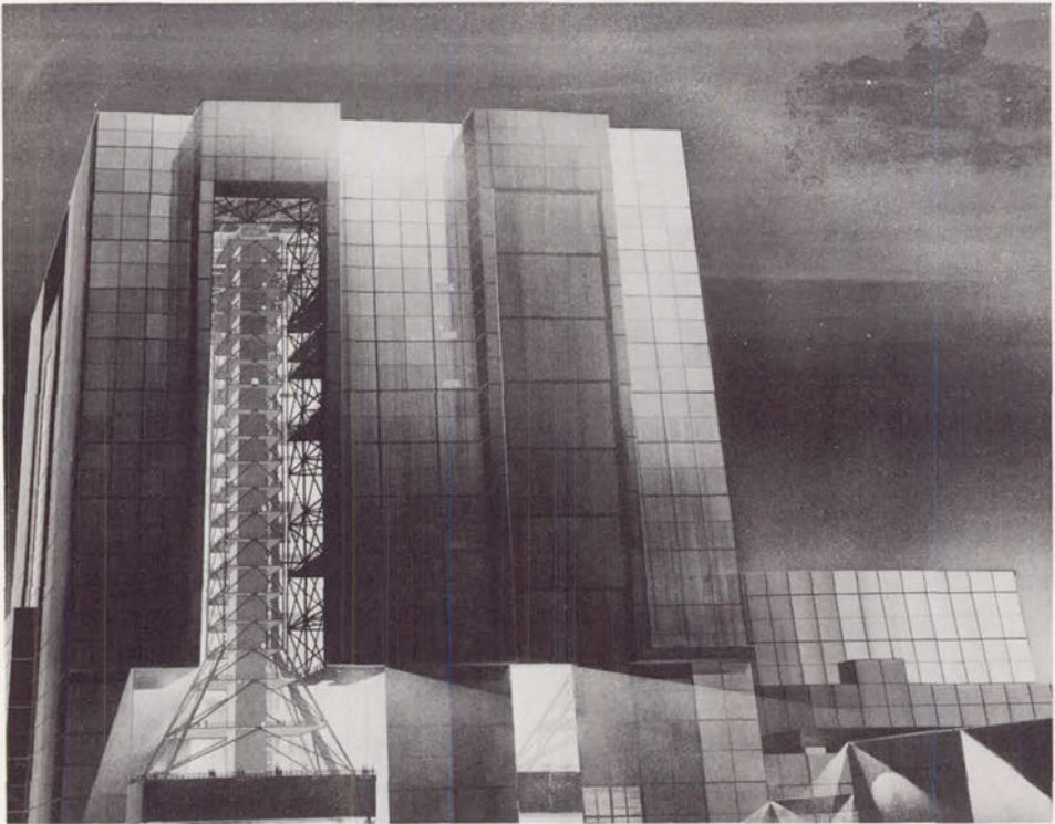
Fig. 57. Sketch of the assembly building, September 1963, showing the doors to the high bays.
