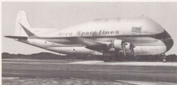
Fig. 47. The Pregnant Guppy, a modified B-377 aircraft used to airlift Saturn stages, July 1963.
