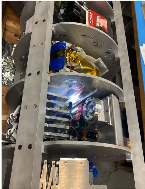
Figure 2-1b: RockSat-X Deck in Longeron Structure (Actual)
