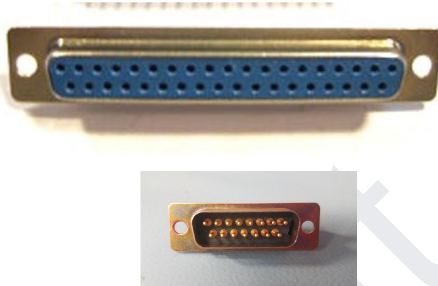
Figure 5-5: Telemetry (Top) and Power (Bottom) Connectors
