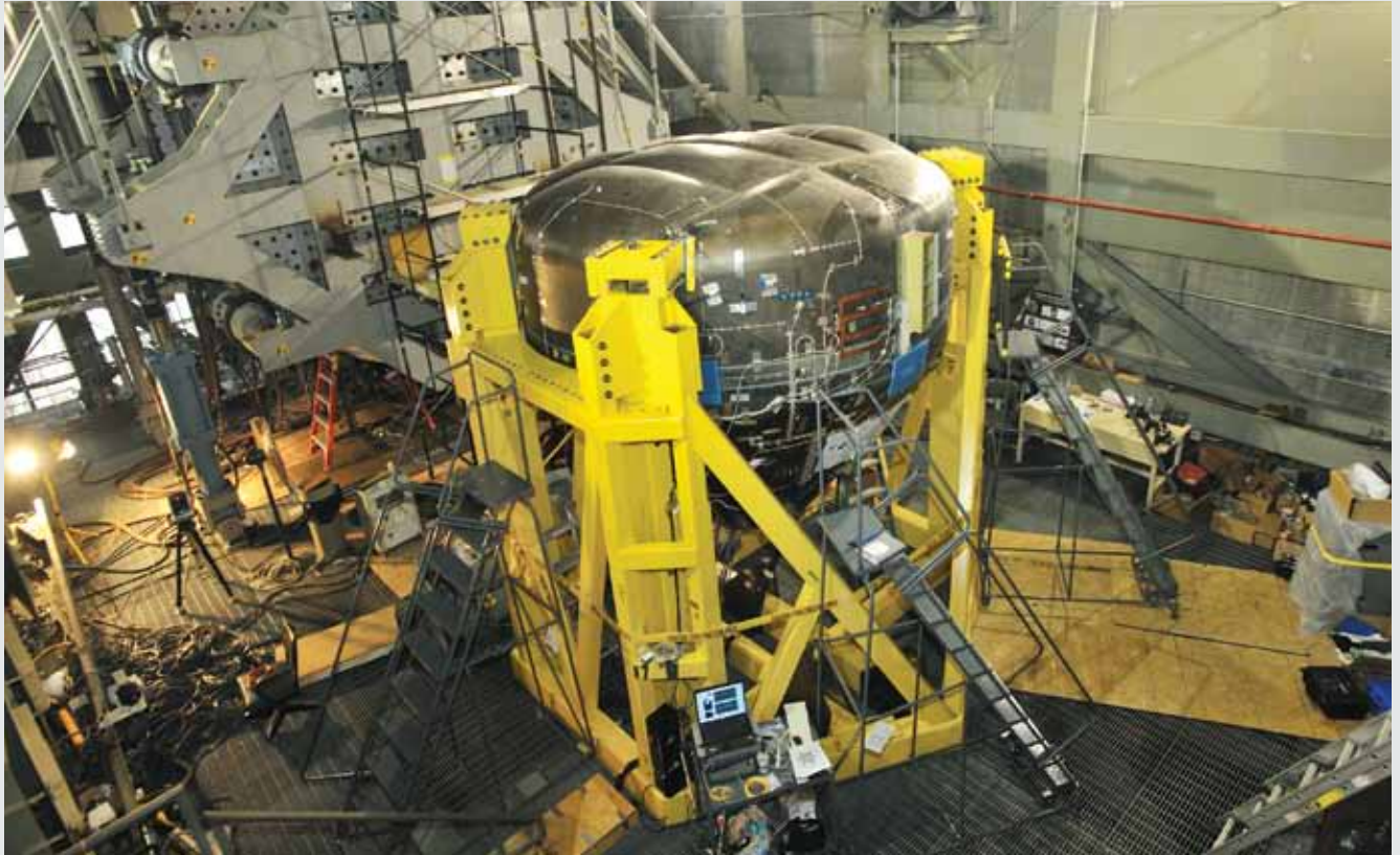
The composite crew module installed in LaRC's Combined Loads Test facility undergoing static internal pressure testing to failure.
