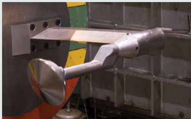
Model of the Mars Science Laboratory mounted in the LaRC 31-inch Mach 10 wind tunnel.
