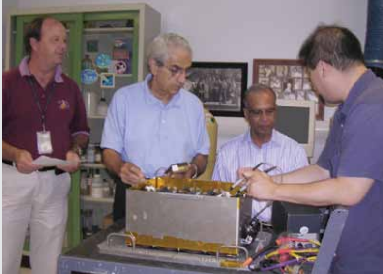
(From left) Denney Keys/NASA Technical Fellow for Electrical Power, Dr. George Dakermanji/MEI, Dr. Hari Vaidyanathan/COMSAT, and Leonine Lee/GSFC Lead Battery Engineer test a spare WMAP CPV NiH2 battery to help assess WMAP in-flight anomalies.
