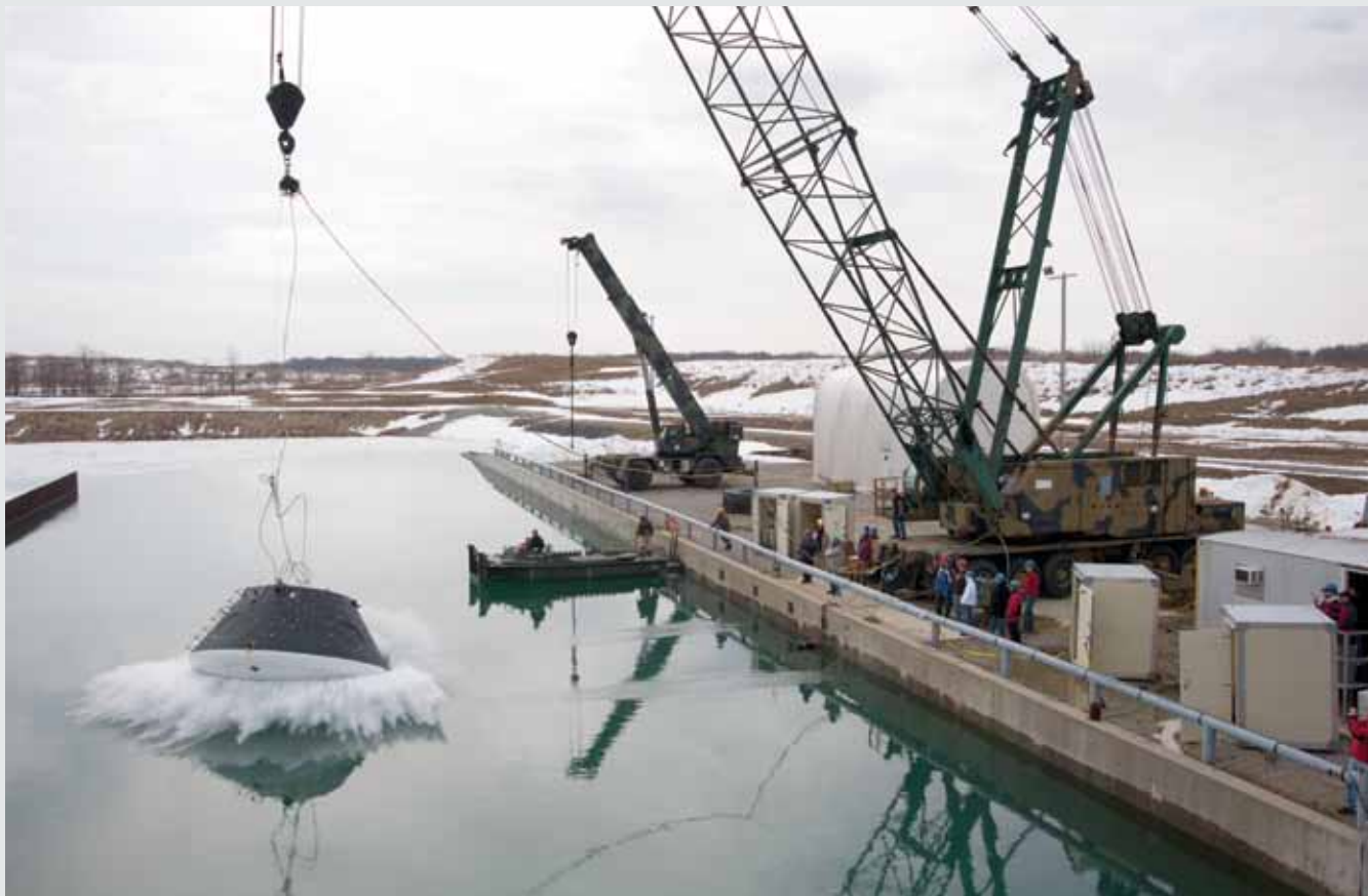
Test drop of an Orion crew module boilerplate to measure the acceleration profile at the vehicle center of gravity. A total of 18 drops were performed at the US Army's Aberdeen Test Center, MD. The CM was previously flown on the Max Launch Abort System Project.
