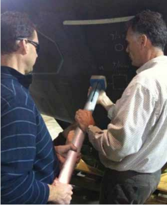
Wade Jackson and Dr. Sotiris Kellas from LaRC delivering impact damage to the CCM using a custom-made impact tool.
