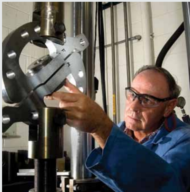
Combined shear/tension testing of aerospace fasteners by James Hodo, Electronics Technician in the Materials and Processing Lab.
