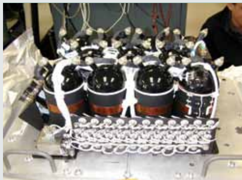
WMAP 23 amp-hr NiH 2 common-pressure-vessel based flight battery during ground acceptance testing prior to launch.
