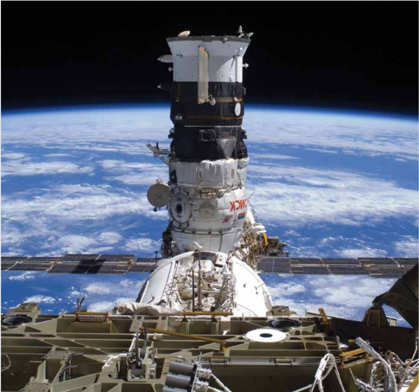
The Russian mini-research module, MRM-2 with Zarya FGB storage module in the foreground.
