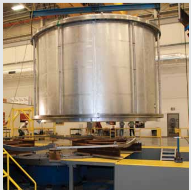
The 27.5-foot-diameter Test Article 1 being installed into the MSFC 7-Axis Milling Machine Facility for the SBKF Project.
