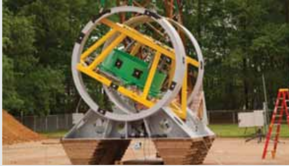
Fullscale seat strut energy attenuation device being tested at NASA Langley Research Center's Landing and Impact Research (LandIR) facility.
