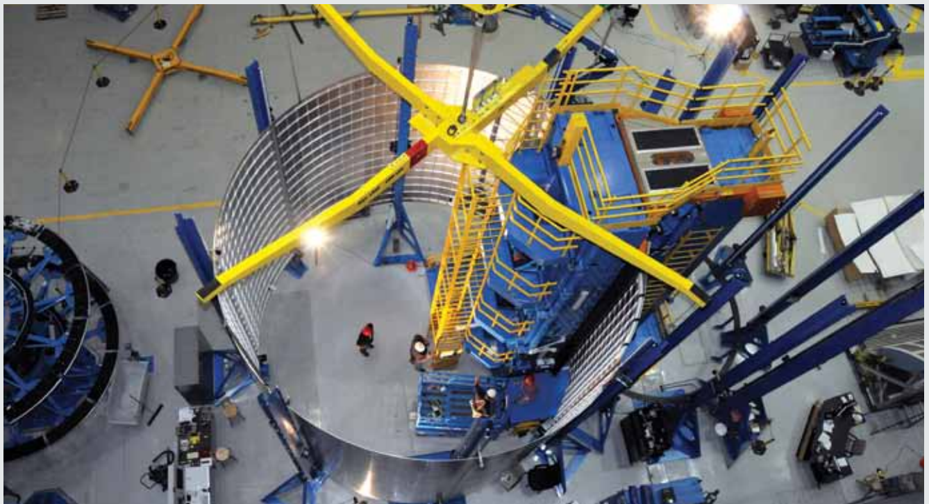
External Tank-derived Test Article 1 in the process of having the final barrel panel welded using the Vertical Weld Tool at MSFC. Each 27.5-foot-diameter by 20-ft-tall barrel is made up of eight individual orthogrid barrel panels and were obtained from the Space Shuttle External Tank Project.
