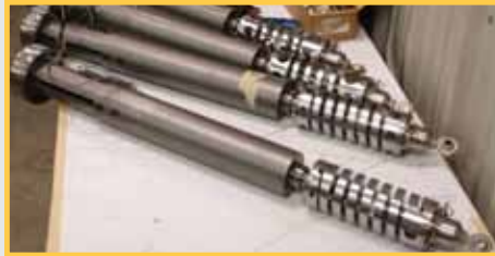
Fullscale seat strut energy attenuation device being tested at NASA Langley Research Center's Landing and Impact Research (LandIR) facility.
