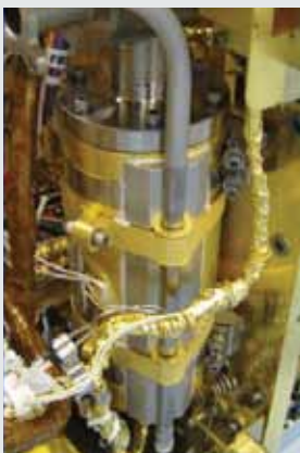
Two Wide Range Pumps are used on the Sample Analysis at Mars instrument to provide vacuum that pulls helium and carbon dioxide gas through the instrument sensors.
