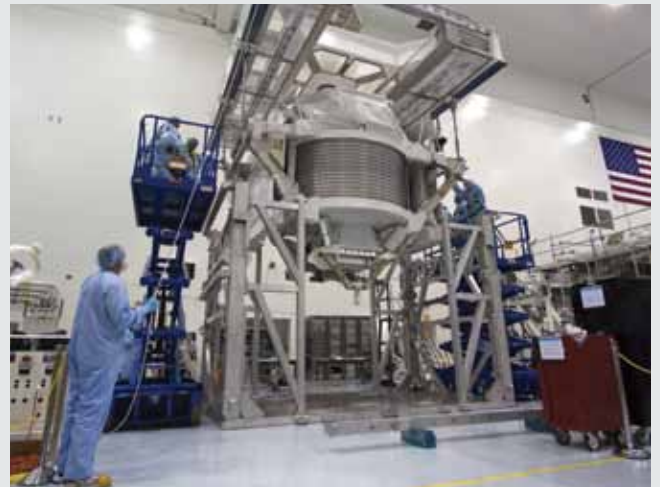
Technicians at KSC's Space Station Processing Facility move AMS-02 from a fixed stand to a rotation stand to begin processing for launch.
