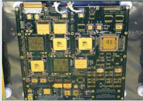
Circuit board using multiple RTAX2000S parts.
