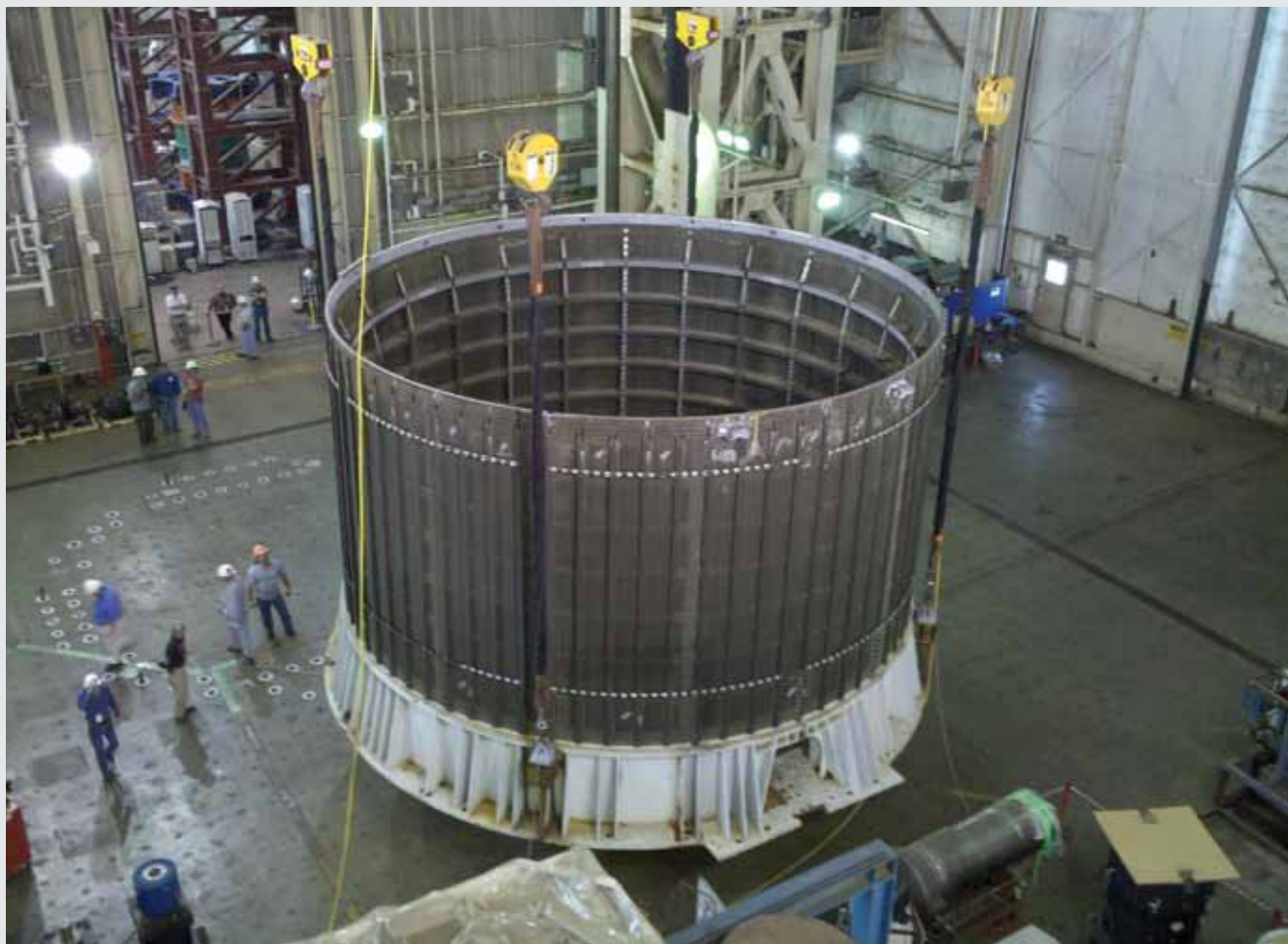
Lower load introduction structure (LIS) in the Loads Test Annex facility at MSFC in preparation for External-Tank-derived Test Article testing (ETTA1).
