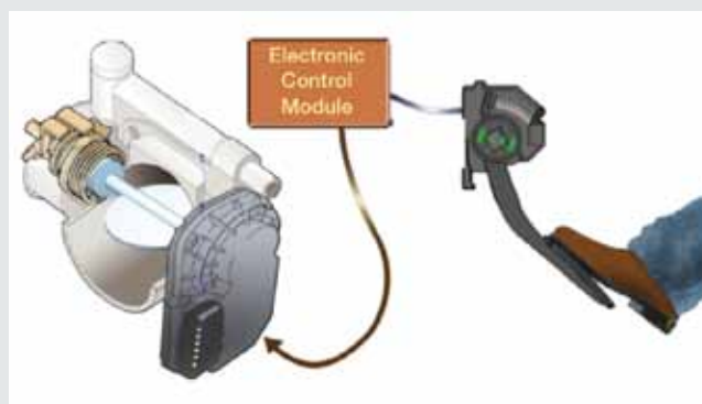
Components of an electronic throttle control which translate pedal position into throttle body opening.
