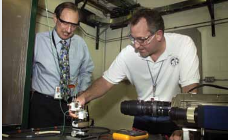
NESC Statistician Ken Johnson (left) observes as Test Conductor Tony Carden (right) aligns the optical pyrometer for temperature measurements of the Y-PCA.
