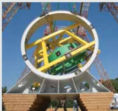
The NESC employed the LaRC's Landing and Impact Research (LandIR) facility to investigate energy attenuating seat struts for the Orion crew module.
