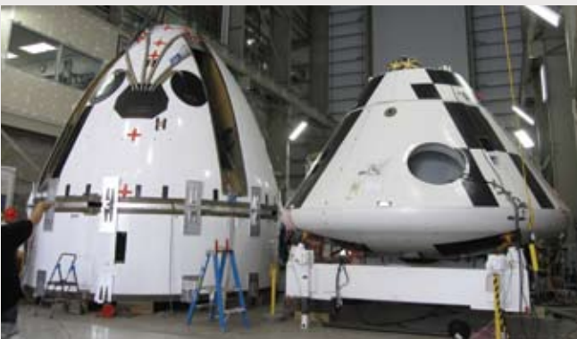
The forward fairing and coast skirt (left) integrated for fit check prior to encapsulation of the crew module (right).
