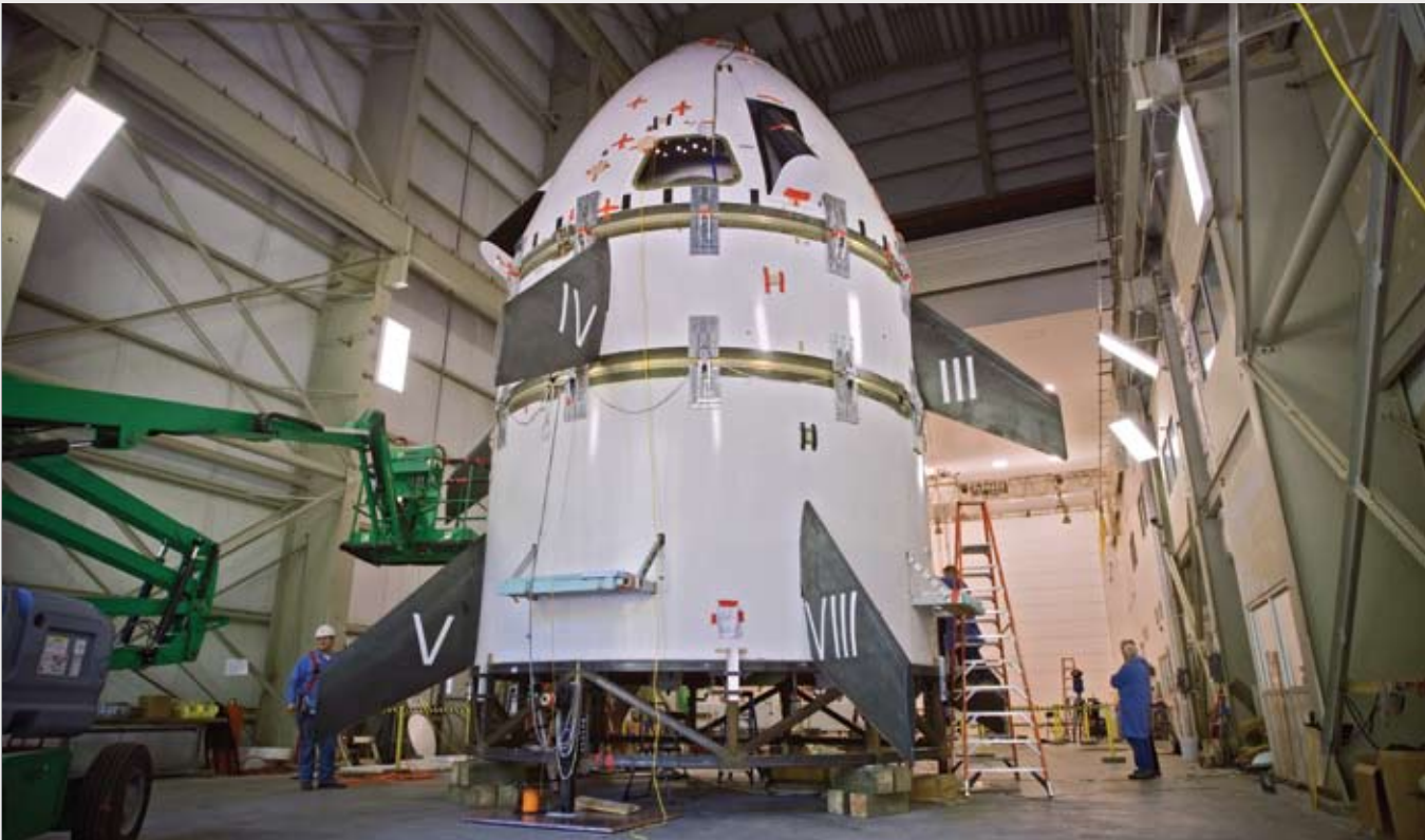
Final check out of the MLAS FTV in the high bay of the WFF Payload Processing Facility prior to transport to the launch pad.
