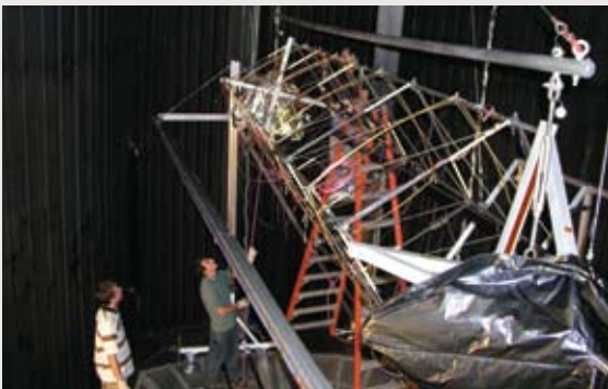
A section of ISS solar array mast was evaluated in the JPL 25-ft Space Simulator to create conditions that could cause buckling of the masts.
