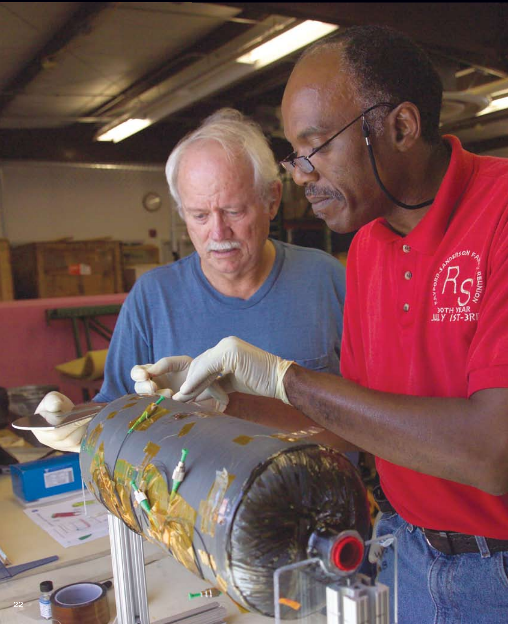
Robert Browning (left) from WSTF and Curtis Banks from MSFC, install conventional and Fiber Bragg Grating strain gauges on a Composite Overwrapped Pressure Vessel for testing.
