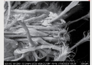
Scanning electron microscopy image showing damaged Vectran™ fibers.
