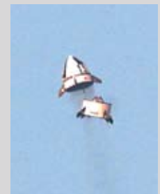
Boost skirt separation viewed from the CM heatshield.
