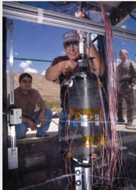
Technician Don Saunders installs a COPV autofrettage test article into the WSTF 860 test system as Project Leader Ralph Lucero (left), Jacobs Technology, looks on.
