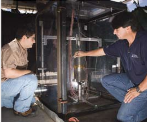
WSTF Project Leader Ralph Lucero (left), Jacobs Technology, and Dr. Valery Godinez, Mistras NDE Solutions, check Acoustic Emission (AE) sensors prior to test.
