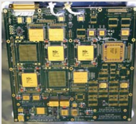
Circuit board using multiple RTAX2000S parts.
