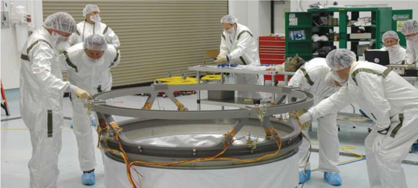
Flight force measurement strain gauges and wiring harnesses can be seen on the Fermi PAF prior to final mating with the booster and Fermi satellite.
