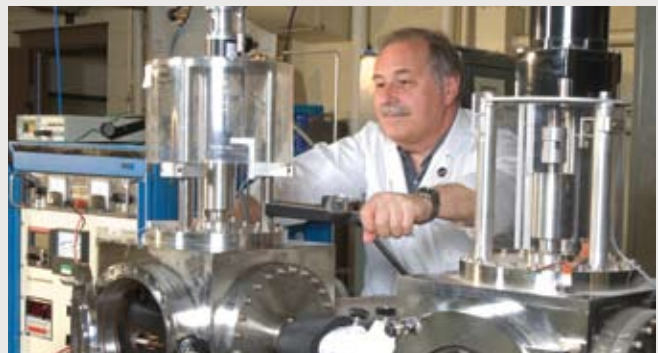
Kenneth Street of the Tribology and Mechanical Components Branch checks initial test conditions for the RWA bearing tests.
