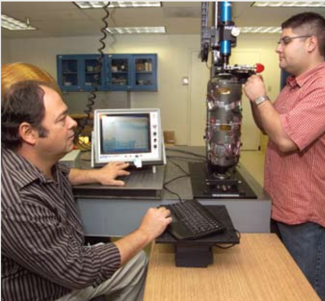
(Above) Tim Gallus (left), MEI Technologies, and Ralph Lucero (right), Jacobs Technology, team up to map the interior of COPVs used in the NESC CPVWG Autofrettage Test Project.
