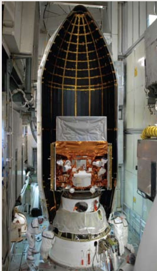
The Fermi satellite stands mated to the Payload Adaptor Fitting inside the mobile service tower on Launch Pad 17-B at Cape Canaveral Air Force Station.
