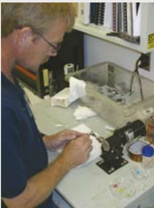
Harold Clayton polishes a flow control valve poppet in preparation for inspection.
