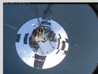
Coast skirt separation viewed from the FTV outer mold line.
