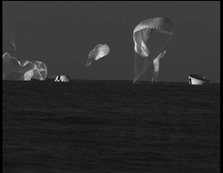
Both visual (left) and infrared (right) imaging of the CM main parachutes provide sufficient detail to assess parachute damage or other operational anomalies.
