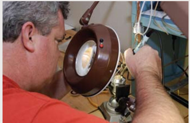
Bob Arp, an aerospace technician with the United Launch Alliance, repairs a replacement feed-through connector installed in the external fuel tank on STS-122.
