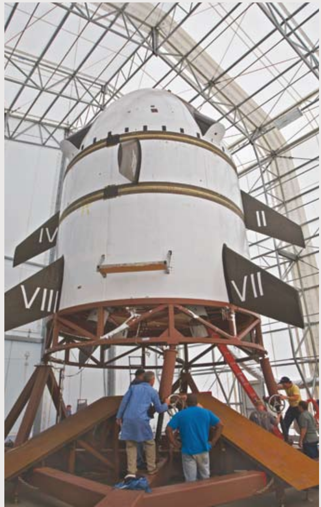
(Above, from left) John Schmalzel, Andrew Bracey, and Stephen Rawls prepare the SiSP sensor package for the MLAS launch. (Right) MLAS Flight Test Vehicle is shown on the launch stool during sensor installation.
