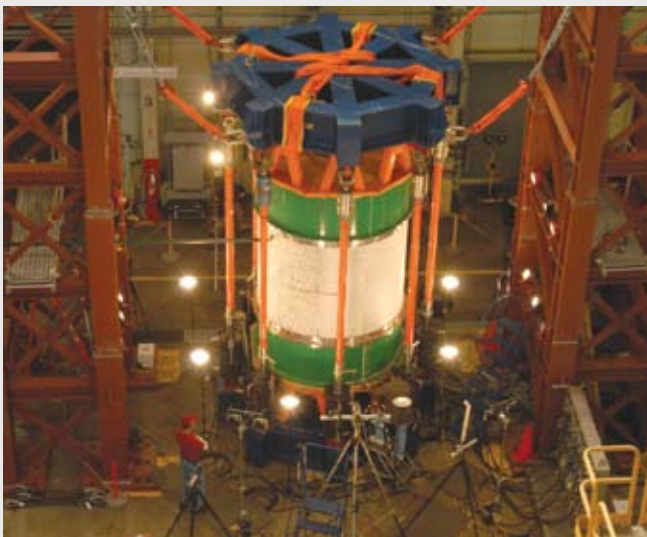
Ares V-style shell undergoing testing at MSFC's Shell Buckling facility.
