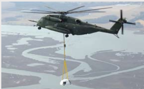
A CH-53 from the HX-21 Air Test and Evaluation Squadron was used to successfully release the MLAS forward bay cover drop test payload.
