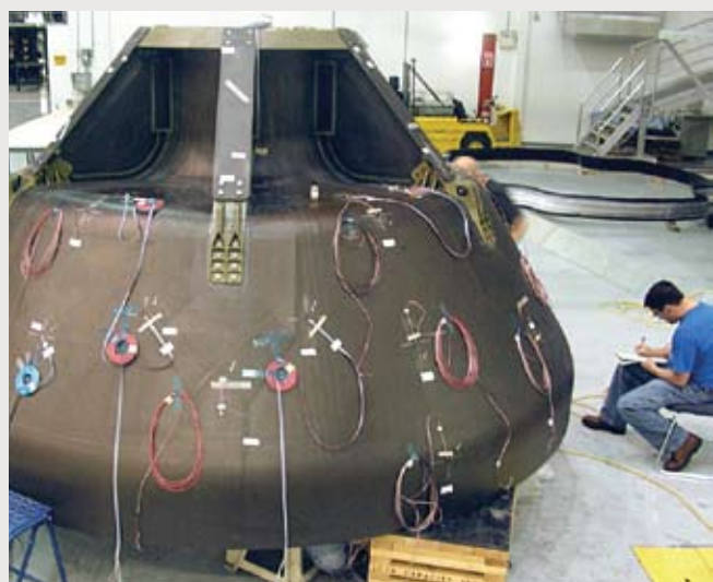
Technicians from the MSFC Test Laboratory installed strain gauges on the CCM and supported testing.
