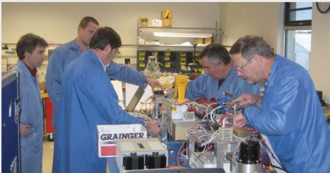
Wallops Flight Facility engineers and technicians assemble the MLAS avionics shown installed in the crew module (shown above).
