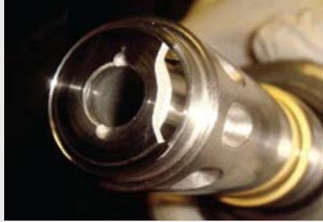
STS-126 orbiter main propulsion system flow control valve poppet fracture showing 20 percent loss of upper flange.
