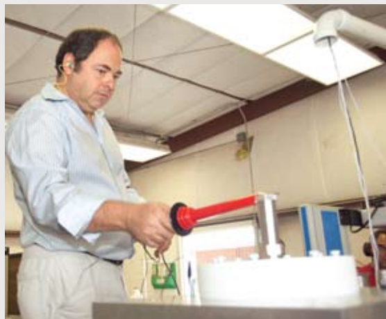
WSTF engineer Tim Gallus measures electrostatic build-up during testing of the TPC. The cartridge is shown installed on the shaker table at the New Mexico State University for vibration testing.
