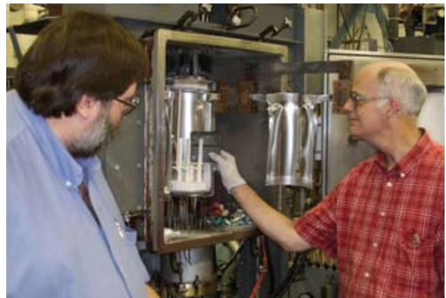
Wallace Vaughn (left) and Craig Ohlhorst (right) examine an RCC test coupon after a high temperature mission simulation cycle in LaRC's Multi-parameter Mission Simulation Facility.
