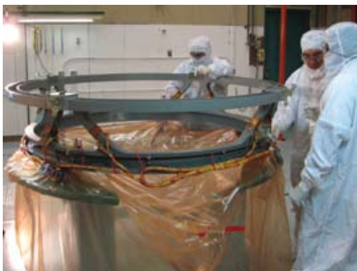
Boeing employees Gerry Darter (left), Henry Fung (center), and Eric Thomas (right) install instrumentation on the GLAST PAF to collect flight force measurements.
