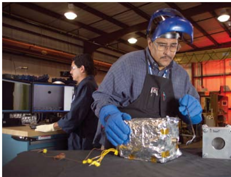
Dennis Garcia, WSTF (right) uses a mirror to view inside the JWST cryogenic box to verify impact on target. Paul Mirabal, WSTF (left) verifies projectile integrity post test on the high speed imaging system.
