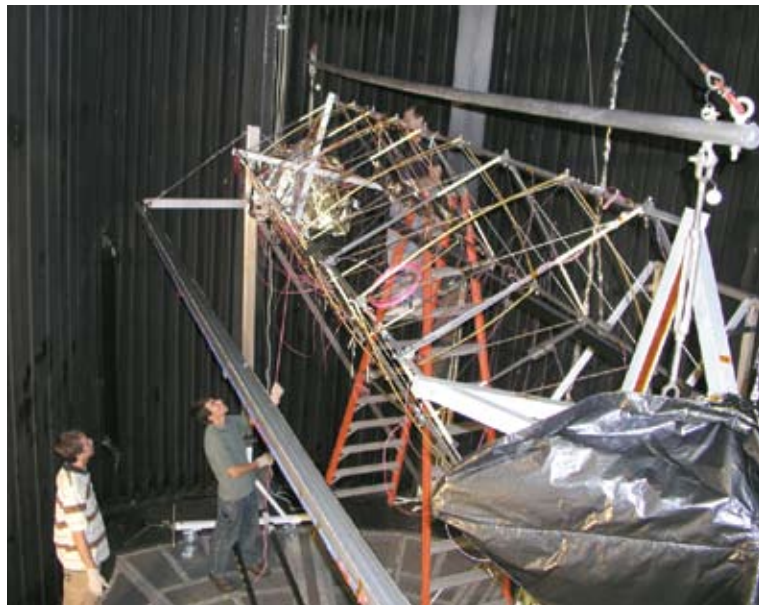
(Above) On orbit, the solar array mast extends, retracts, and provides structural support for the solar array panels.
