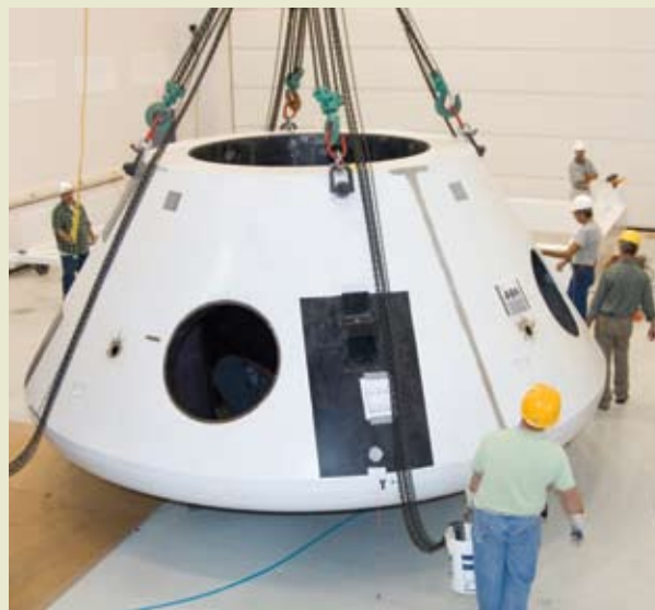
The full scale Orion Crew Module simulator being prepared for mass properties measurements.
