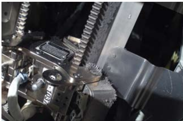
Magnetized debris seen on the SARJ trundle bearing assembly. Twelve trundle bearing assemblies are equally spaced around the circumference of the SARJ and provide precision support and alignment during rotation of the SARJ.
