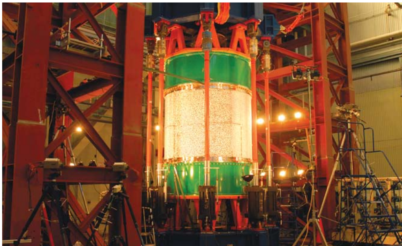
New Shell Buckling Test Facility at MSFC used for testing 8-ft-diameter cylinders subjected to combined compression, bending and internal pressure.
