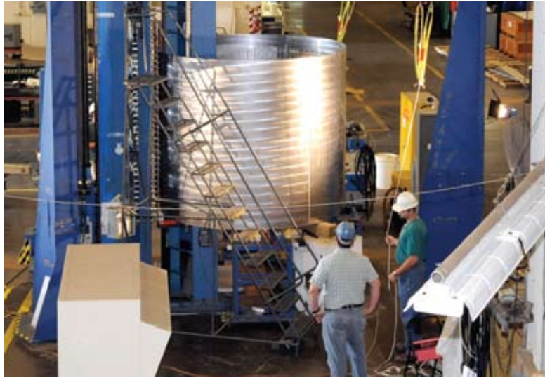
Orthogrid panel segment welded into a barrel section in the Vertical Weld Tool for the Shell Buckling Knockdown Factor work.
