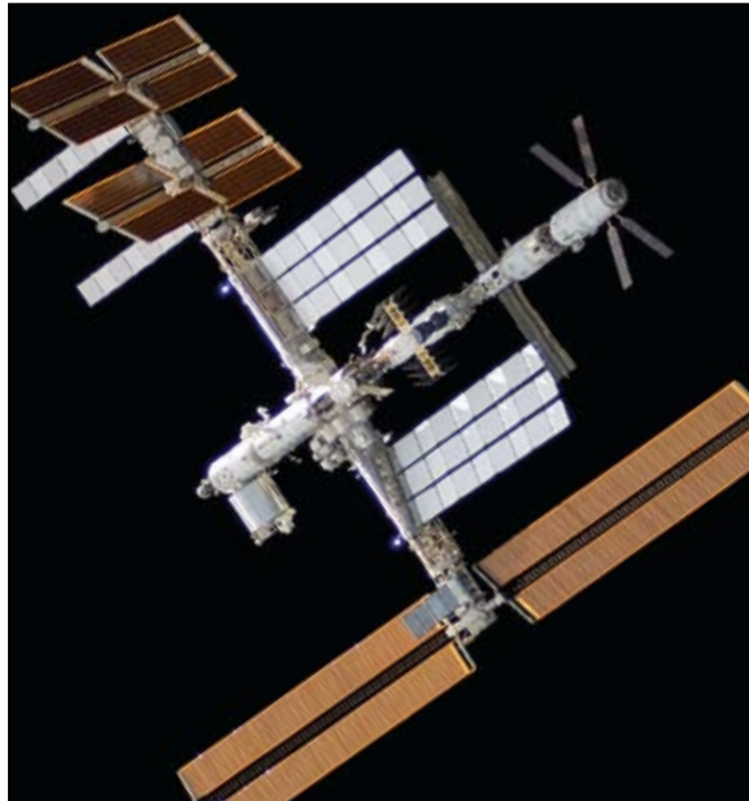
One major component of the International Space Station (ISS) remains to be installed. S6 contains the fourth and final set of solar arrays and batteries.
