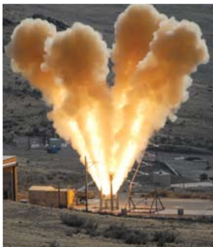
The NASA and Orion industry team conducted a successful test firing of the LAS abort motor.
