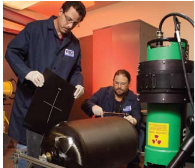
Ben Gonzalez, GeoControl Systems Inc., and Brooks Wolle, Jacobs Technology Inc., perform radiograph inspection of COPV weld anomalies at WSTF.
