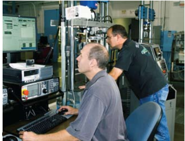
Dr. David Dawicke and Greg Shanks conduct fracture tests on welded A516 Steel for critical initial flaw sizes (CIFS) in USS segments for Ares I-X
