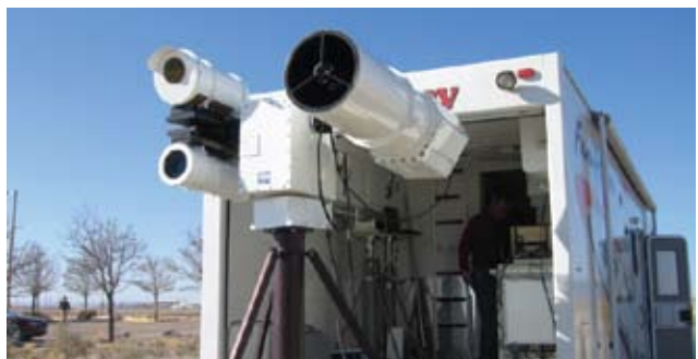
Mobile Aerial Tracking and Imaging System (MATRIS) set up to support the HYTHIRM calibration test at Sandia National Laboratory's Solar Tower.
