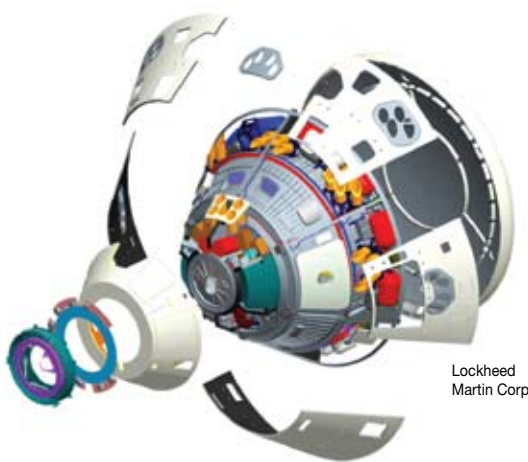
The number of parts on the Crew Exploration Vehicle, Orion, and other CxP components requires accurate knowledge of mass properties and its effects on the vehicle's performance.
