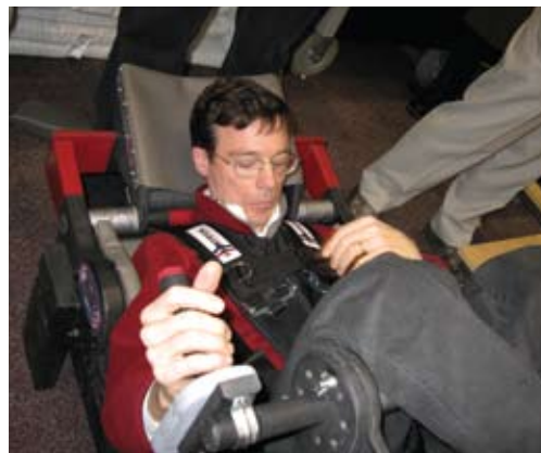
NESC team member Pete Rossoni performs a fit check in an Orion seat mock-up at JSC.
