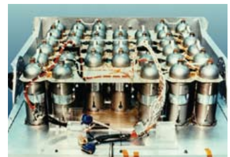
(Above) The Battery Working Group meets to work issues with existing batteries and to develop next generation batteries. (Right) GRC developed and validated designs for nickel hydrogen (Ni-H 2 ) cells that have been adopted for NASA missions and employed by cell manufacturers and satellite companies.
