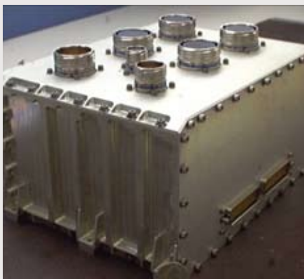
The Phoenix Pyrotechnic Initiation Unit sends current pulses of precise magnitude and duration to the NASA Standard Initiators on the Phoenix spacecraft to start numerous actions.
