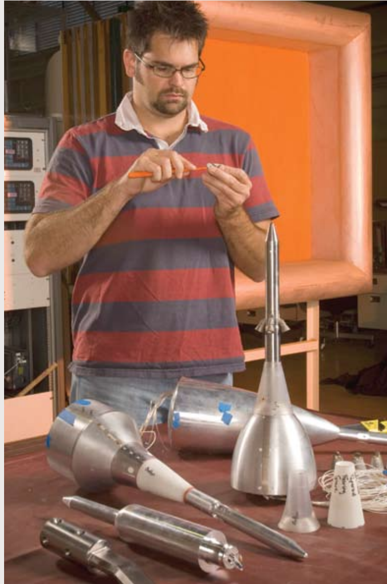
Nate Burnside, ARC's Principal Investigator of the Fluid Mechanics Laboratory, cleans a nozzle after the 50-AS testing was completed. The baseline 605-068 LAV, ALAS-2, and ALAS-11 models are in the foreground.
