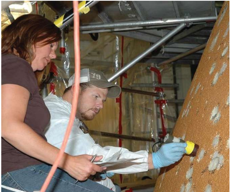
United Space Alliance personnel, Nancy Lewis and Jessie Lawhorn, repair damage to the External Tank's foam insulation caused by hail damage while Atlantis was on the launch pad at KSC.
