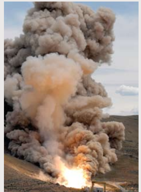
The plume diagnostic engineers at SSC measured the heat flux from the plume of a Space Shuttle solid rocket motor during a test firing.
