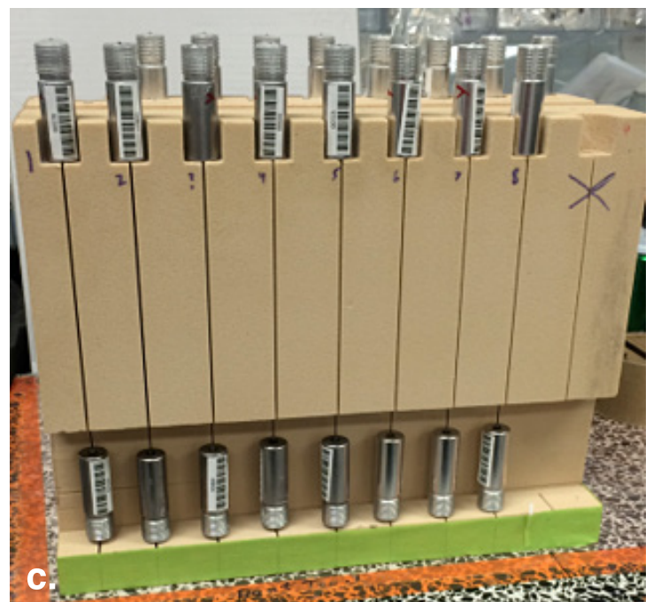
To gather strand stress rupture data, a team at MSFC fabricated strand specimens by impregnating carbon fibers with resin, threading them through shrink-fit tubing, and curing them in an oven (a). At LaRC, grips were applied and the strands (b), and completed test specimens were tested at WSTF (c).
