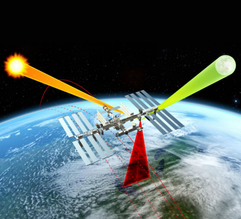
An illustration of how CLARREO Pathfinder will take measurements of Earth (red) and use the Sun (orange) and Moon (green) for regular instrument calibration on ISS.
