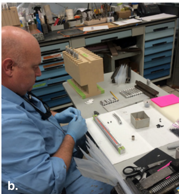
To gather strand stress rupture data, a team at MSFC fabricated strand specimens by impregnating carbon fibers with resin, threading them through shrink-fit tubing, and curing them in an oven (a). At LaRC, grips were applied and the strands (b), and completed test specimens were tested at WSTF (c).
