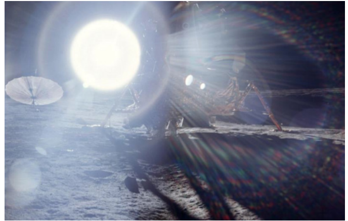
Apollo 12; the lander with the sun in the field of view, illustrating the challenges to functional vision (the photographic flare does not represent the actual size of the sun). In Artemis landings, the sun will always be below this elevation.
