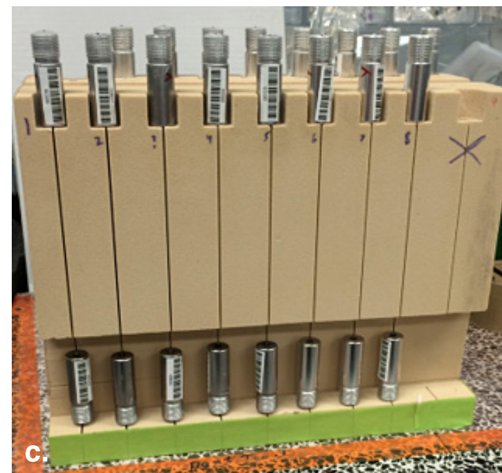
To gather strand stress rupture data, a team at MSFC fabricated strand specimens by impregnating carbon fibers with resin, threading them through shrink-fit tubing, and curing them in an oven (a). At LaRC, grips were applied and the strands (b), and completed test specimens were tested at WSTF (c).
