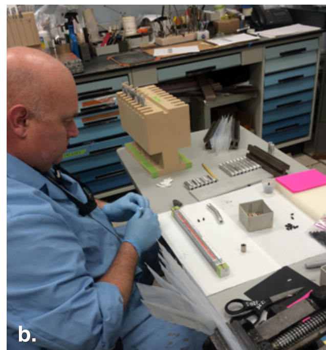
To gather strand stress rupture data, a team at MSFC fabricated strand specimens by impregnating carbon fibers with resin, threading them through shrink-fit tubing, and curing them in an oven (a). At LaRC, grips were applied and the strands (b), and completed test specimens were tested at WSTF (c).
