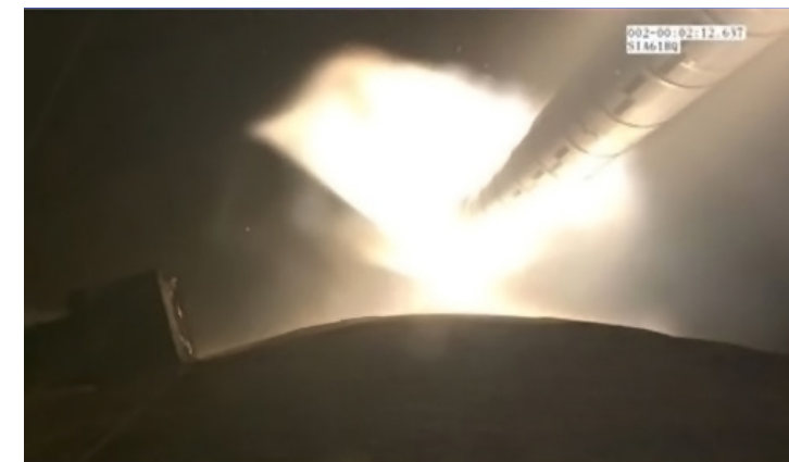
These figures compare frames from the NESc simulation to the Artemis I flight imagery at 1.86 seconds after SRB separation, when the near-field separation clearances are critical. Analysis results supported the SLS Program's conclusion that the SRB separation event was nominal and separation clearances were as expected.
