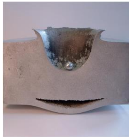
Figure 2. Impact crater from 1.2 cm aluminum sphere traveling at 6.8 km/s striking 18 cm thick block of aluminum. Source NASA ODPO.
