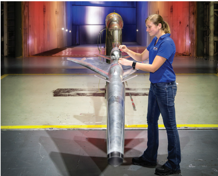
Engineer Samantha O'Flaherty with a supersonic airplane model in a wind tunnel.
