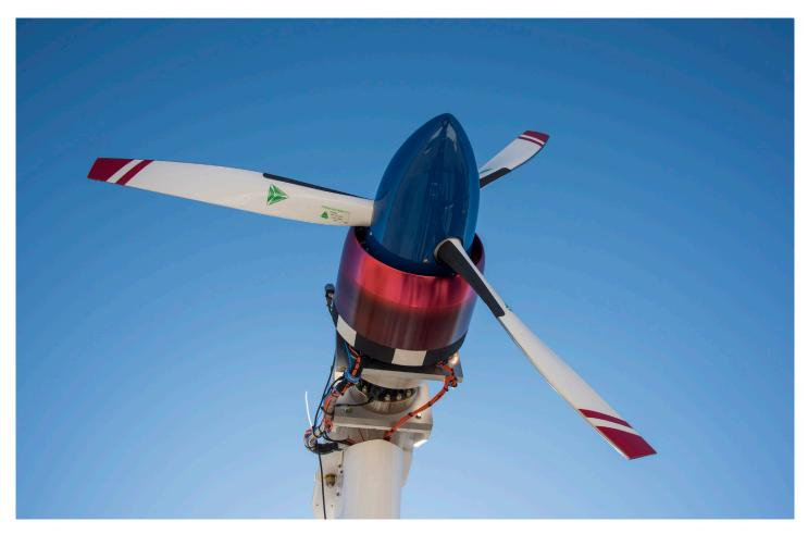
A JM-X57 cruise motor, designed and built by Joby Aviation in Santa Cruz, California, sits in its test position on the Airvolt test stand at NASA Armstrong Flight Research Center in California. Extensive testing is necessary to validate the motor system's safety and functionality in order to be deemed flightworthy according to NASA's flight qualification process. X-57 will be NASA's first all-electric X-plane.
