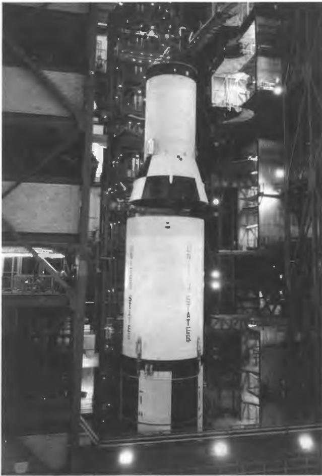
Apollo 11 third stage (S-IVB) is being raised for mating to the second stage. NASA Photo #69-H-321.
