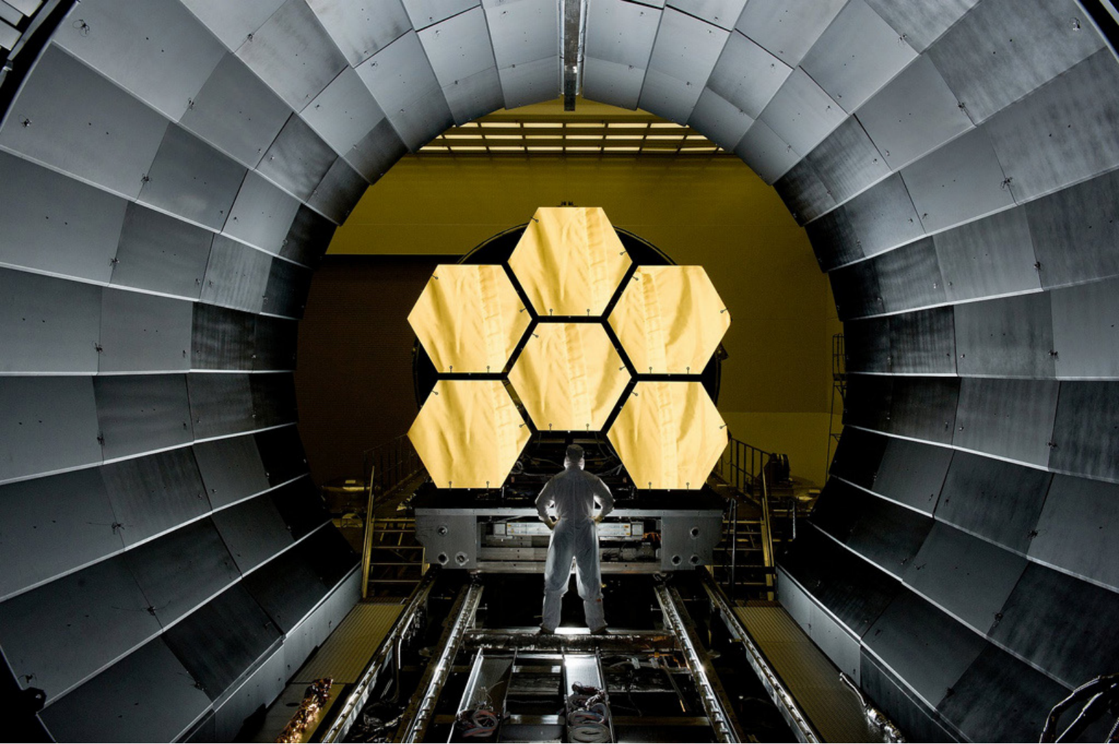
The first six of 18 segments that will form NASA's James Webb Space Telescope's primary mirror for space observations begin the final round-the-clock cryogenic testing. These tests will confirm the mirrors will respond as expected to the extreme temperatures of space prior to integration into the telescope's permanent housing structure. Photo credit: NASA/MSFC/David Higginbotham
