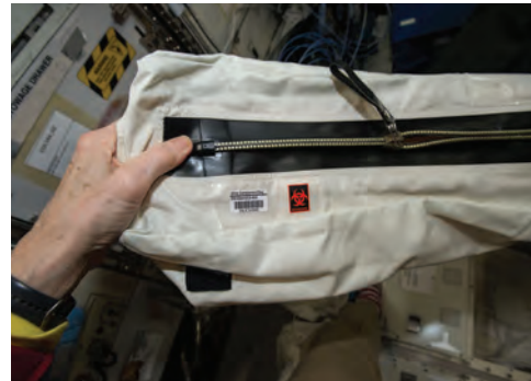
Figure 81. UCB, used for holding discarded UCDs until they can be disposed of along with other trash from the ISS. Photo Credit: NASA.
