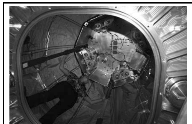
Bigelow Aerospace Integration Engineer Sofia Russ stands inside the Bigelow Expandable Activity Module (BEAM) qualification unit after successful testing in preparation for flight in 2015. BEAM is a human-rated, expandable habitation structure utilizing the International Space Station to conduct fundamental research on performance of expandable modules in the space environment.
