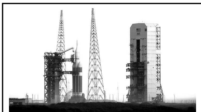
NASA's Orion spacecraft sits on the pad atop a Delta IV Heavy rocket prior to the December 5th launch of Exploration Flight Test-1 from Kennedy Space Center. The two orbit flight sent Orion 3,600 miles into space – farther than any human space flight vehicle since the Apollo 17 mission in 1972.
