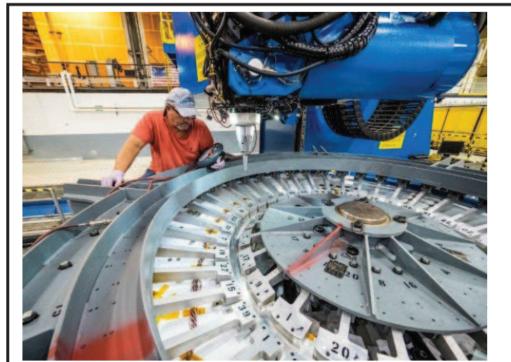
Engineers at NASA's Michoud Assembly Facility (MAF) in New Orleans, LA, perform the first weld on the Orion spacecraft pressure vessel for EM-1 on Sept. 5, 2015. This is the third Orion pressure vessel built. Engineers continue to refine the design, reducing the number of welds from 33, on the first pressure vessel, to seven on the current one, saving 700 pounds of mass.
