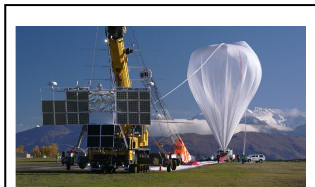
The COSI payload shortly before launch from Wanaka, NZ on May 16, 2016. During the 46-day flight of the super-pressure balloon, COSI observed the gamma-ray emission from our Milky Way galaxy and detected a gamma-ray burst on May 30, 2016.
