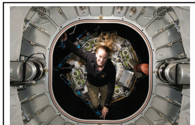
NASA astronaut Kate Rubins inspected the Bigelow Aerospace Expandable Activity Module (BEAM) attached to ISS. Expandable habitats are designed to take up less room on a spacecraft while providing greater volume for living and working in space once expanded. BEAM is the result of a public-private partnership that allowed Bigelow to deploy and test this capability at a fraction of the cost.
