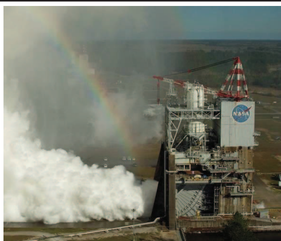
This aerial picture shows the successful RS-25 hot-fire test conducted February 22, 2017 at Stennis Space Center's A1 test stand. Four RS-25 engines along with two, five-segment solid rocket boosters, will power the SLS on missions to deep space. The ongoing testing of the RS-25 engine provides critical data on the newly designed Engine Controller Unit.
