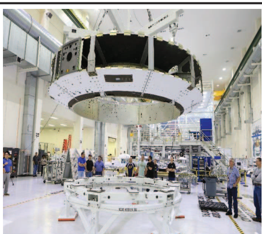
The Orion crew module adapter was lifted out of its work stand Nov. 11 and is now undergoing secondary structure outfitting in the Neil Armstrong Operations and Checkout Building high bay at NASA's Kennedy Space Center in Florida. Photo credit: NASA/ Glen Benson
