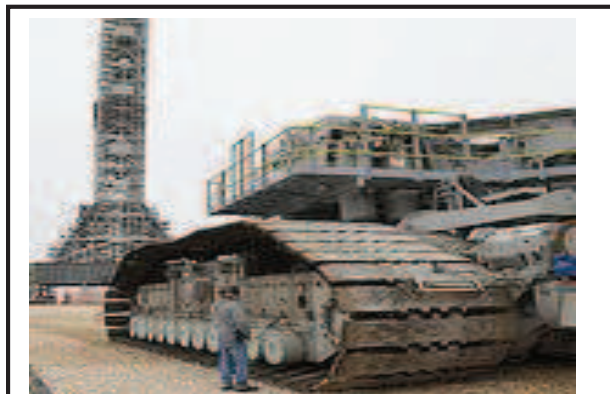
A technician monitors the progress as NASA's Crawler-Transporter 2 moves slowly along the crawlerway back to the crawler park site after a test run to LC-39B at NASA's KSC in Florida. Upgrades to the crawler include 88 new roller bearings, 22 on each "truck" section, and a new jacking, equalizing and leveling system. (In the background is the new mobile launcher.)
