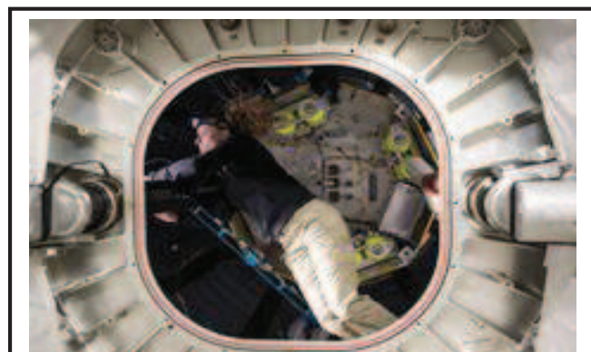
The Bigelow Expandable Activity Module (BEAM) is the first expandable habitat to be installed on the space station. It was expanded on May 28, 2016. Expandable habitats are designed to take up less room on a spacecraft, but provide greater volume for living and working in space once expanded. Astronaut Kate Rubins conducted several evaluations inside BEAM, including air and surface sampling.
