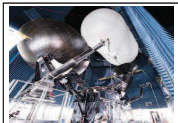
The Tracking and Data Relay Satellite (TDRS-M) is undergoing final testing before its scheduled launch in August 2017 from Cape Canaveral, Florida. The geosynchronous fleet of TDRS is the space segment of the Space Network and operates 24 hours a day, 7 days a week. It provides communication and tracking services to missions in low Earth orbit.
