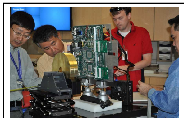
NASA's Electronic Parts and Packaging (NEPP) is leading a government/industry/academia team evaluating electronics radiation testing for space applications. This research is being conducted at the SCRIPPS Proton Therapy Center and includes representatives from the Air Force, NRO, Boeing, Vanderbilt University, and SpaceX.
