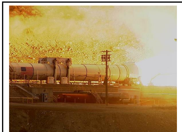
At the Promontory, Utah test facility of Orbital ATK, the booster for NASA's SLS rocket fired for a two-minute test on March 11, 2015. NASA and Orbital ATK have successfully completed three full-scale development test firings of the five-segment solid rocket motor, as well as the important booster CDR)
