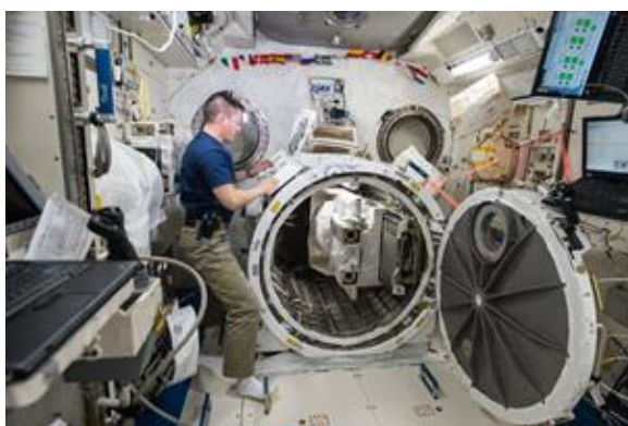
NASA astronaut Kjell Lindgren loads a deployer device filled with 16 CubeSats into a small airlock in the Japanese Kibo Module on the ISS. Among the 16 satellites are 14 Dove satellites from Planet Labs that will be used for Earth observation, one for testing space based radios and another that will be used to track ships on the open ocean.
