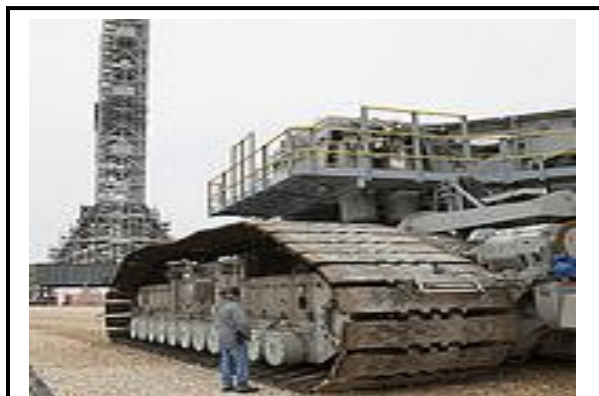
A technician monitors the progress as NASA's crawler-transporter 2 moves slowly along the crawlerway back to the crawler park site after a test run to Launch Pad 39B at NASA's KSC in Florida. Upgrades to the crawler include 88 new roller bearings, 22 on each "truck" section, and a new jacking, equalizing and leveling system. In the background is the new mobile launcher.)
