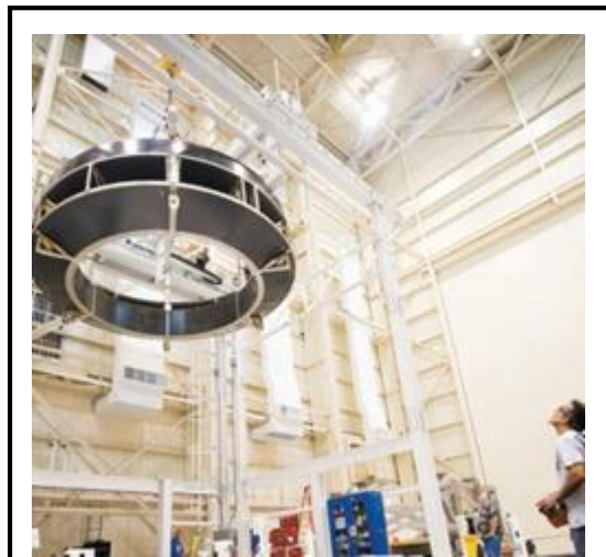
Lockheed Martin technicians lift the Orion Crew Module Adapter Structural Test Article at NASA Glenn Research Center (GRC)' s Plum Brook Station. The adapter will connect Orion's crew module to a service module provided by the European Space Agency (ESA) and Airbus Defense & Space.
