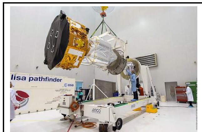
The Laser Interferometer Space Antenna (LISA) Pathfinder mission undergoes preparations ahead of its launch from Kourou, French Guiana. NASA is contributing the Space Technology (ST) 7, which will use precision microthrusters to demonstrate that a solid body can float freely in space completely undisturbed. Credit: ESA-CNES-Arianespace/Optique.
