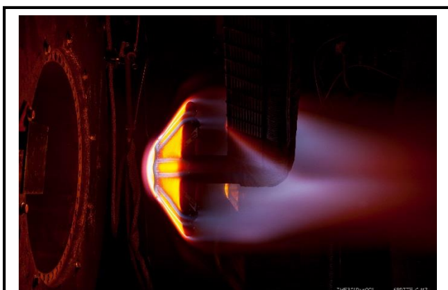
Heating simulation testing of an Adaptive Deployable Entry and Placement Technology model under conditions akin to entering the Martian atmosphere at the Arc Jet Complex, located at NASA’s ARC, Moffett Field, California. The Arc Jet Complex is used to simulate the aerothermodynamic heating that a spacecraft endures throughout atmospheric entry. NASA’s unique aerothermodynamic testing capability is critical to the design, development, and qualification of spacecraft thermal protection systems (TPS) for space exploration and scientific missions.
