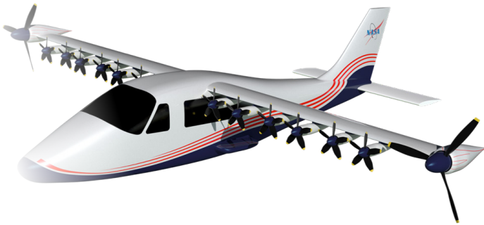
NASA's X-57 is an all-electric experimental aircraft designed to demonstrate multiple leading-edge technologies.
