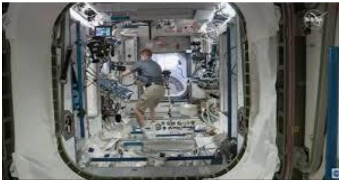
View through Lab forward Node 2 (N2) aft hatches looking forward. Note N2 forward hatch and PMA-2 visible in center of image.
