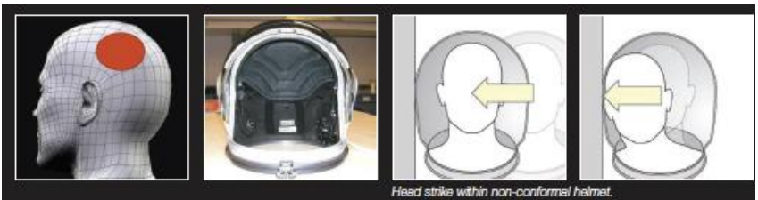
Figure 2.7. Impact injury caused by non-conformal helmet. Image courtesy of Biodynamics Research Corporation, reproduced from Loss of Signal (Stepaniak et. al. 2014).
