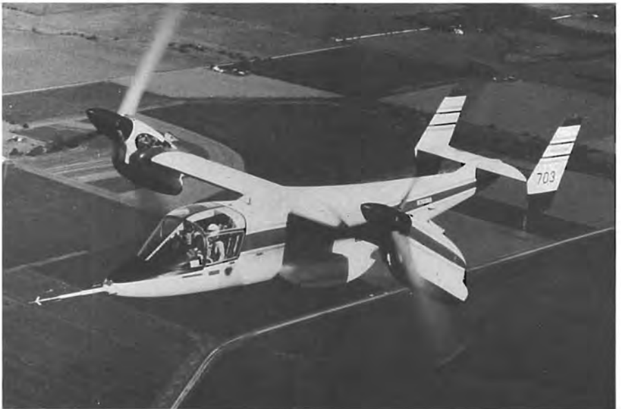
The XV-15 tilt rotor research aircraft. For takeoff (above), the craft's rotors are horizontal to provide lift, then they pivot forward (bottom) to a full vertical position to give cruising speeds twice those of conventional helicopters.
