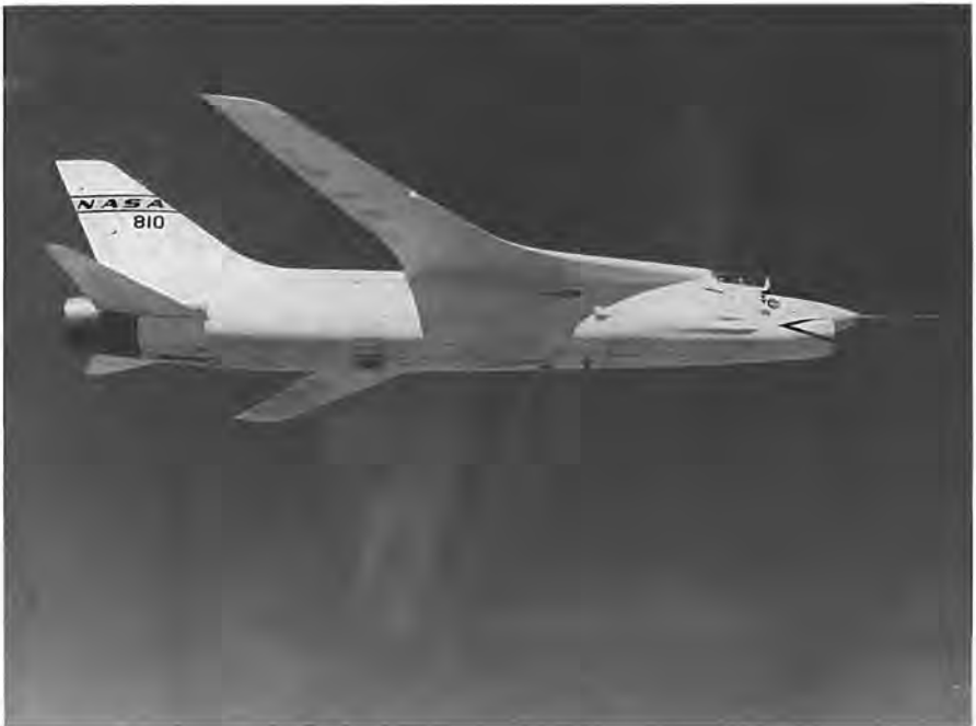
The TF-8A research airplane with its modified supercritical wing.
