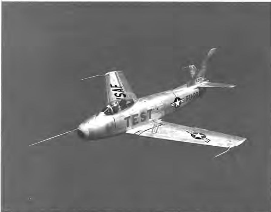
The North American F-86 Sabre featured swept wing and tail surfaces. The plane shown here was fitted with special instrumentation for transonic flight research conducted by the Ames Laboratory.
