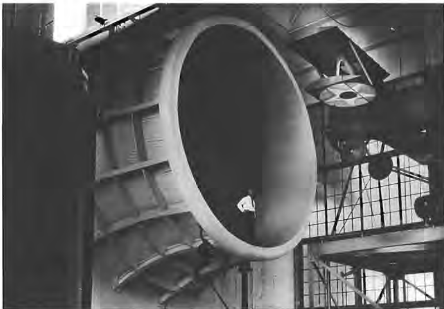
A Sperry Messenger mounted for testing in Langley's propeller research tunnel in 1927.
