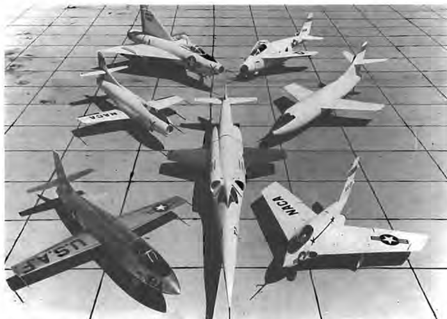
This group portrait displays typical high-speed research aircraft that made headlines at Muroc Flight Center in the 1950s. The Bell X-1A (lower left) had much the same configuration as the earlier X-1. Joining the X-1A were (clockwise): the Douglas D-558-I Skystreak; Convair XF92-A, Bell X-5 with variable sweepback wings, Douglas D-558-II Skystreak; Northrop X-4; and (center) the Douglas X-3.
