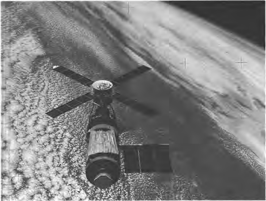
Mission accomplished, the Skylab orbital sails serenely above cloud-covered Earth in this photo taken by the last crew as they leave to return to Earth. The mission-saving emergency shroud shows clearly against the dark surface of the vehicle.
