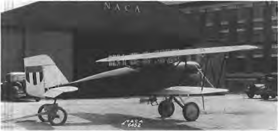
The NACA cowling, as fitted on a Curtiss Hawk, a standard U.S. Army combat plane.
