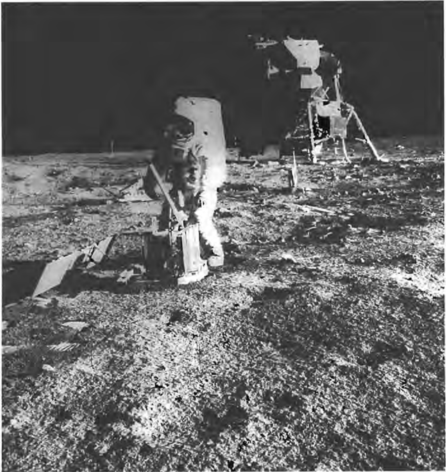
Astronaut Neil A. Armstrong took this photograph of Edwin E. Aldrin, Jr., deploying the passive seismic experiments at Tranquility Base, while ungainly lunar module crouches in the background.
