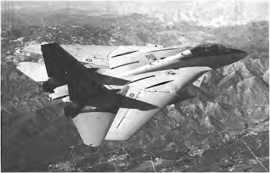
The Grumman F-14 Tomcat, with wings swept back for high-speed flight, was a legacy of variable geometry studies (photo courtesy of Grumman Aerospace Corporation).
