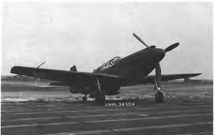
The NACA's laminar flow airfoil was first used on the North American XP-51 Mustang.
