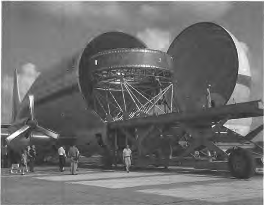
As manned space launches became more frequent, logistics became a major problem. Oversized cargoes like the Apollo instrument unit segment, as well as command modules and upper stages were carried by the Super Guppy, a dramatically modified Boeing Stratoliner.
