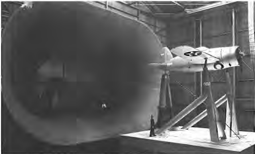
Drag reduction studies on the Brewster XF2A-1 Buffalo influenced many later military fighters.
