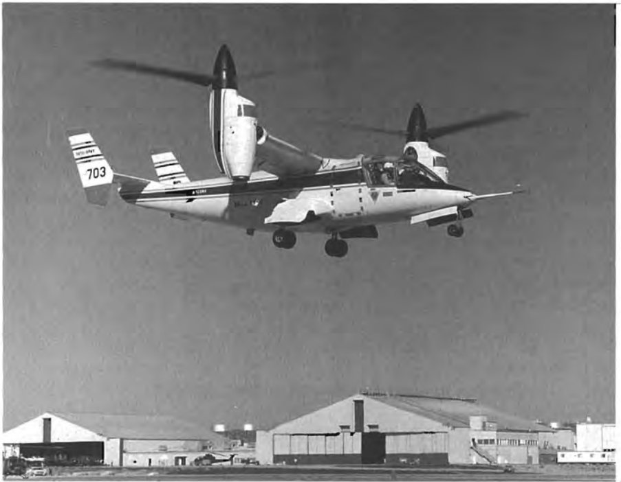
The XV-15 tilt rotor research aircraft. For takeoff (above), the craft's rotors are horizontal to provide lift, then they pivot forward (bottom) to a full vertical position to give cruising speeds twice those of conventional helicopters.
