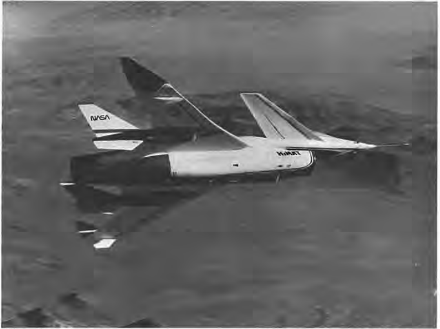
The Highly Maneuverable Aircraft Technology test model (HiMAT), shown during a test flight. A modular design allowed engineers to test a variety of wings, control surfaces, and different structural materials.
