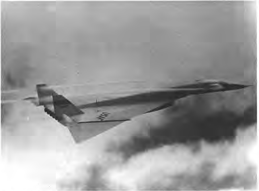
The North American XB-70 yielded valuable data on flight characteristics of large, supersonic aircraft. This photo of a test flight shows shock waves and vortices forming on the fuselage and wings.
