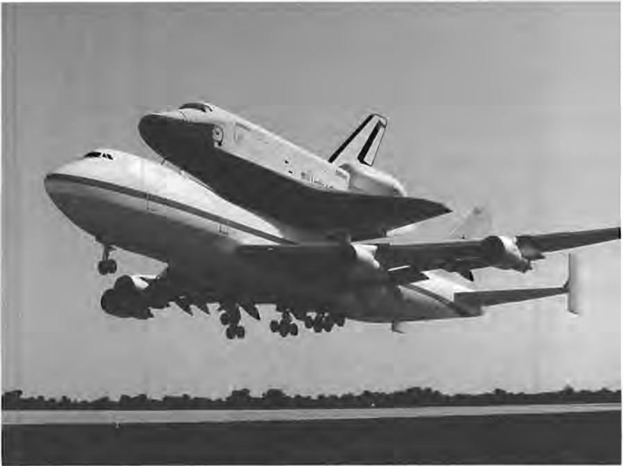
The Shuttle orbiter's descent/landing tests were launched from the Boeing 747, also used to carry orbiters between Kennedy, Edwards Air Force Base, and other sites.
