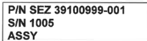
Figure 6: Example of identification markings on hardware that is part of an assembly
