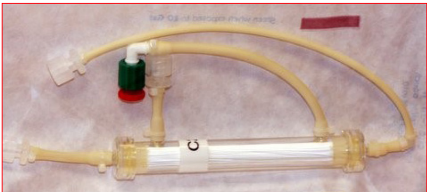
Figure 13: A Single bioreactor unit removed from a bioculture system cassette.
