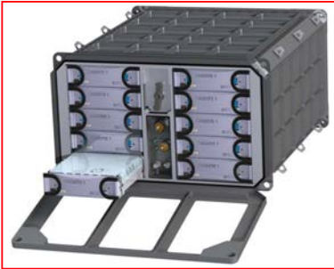
Figure 10: The BioCulture System with ten independent, removable cassettes.
