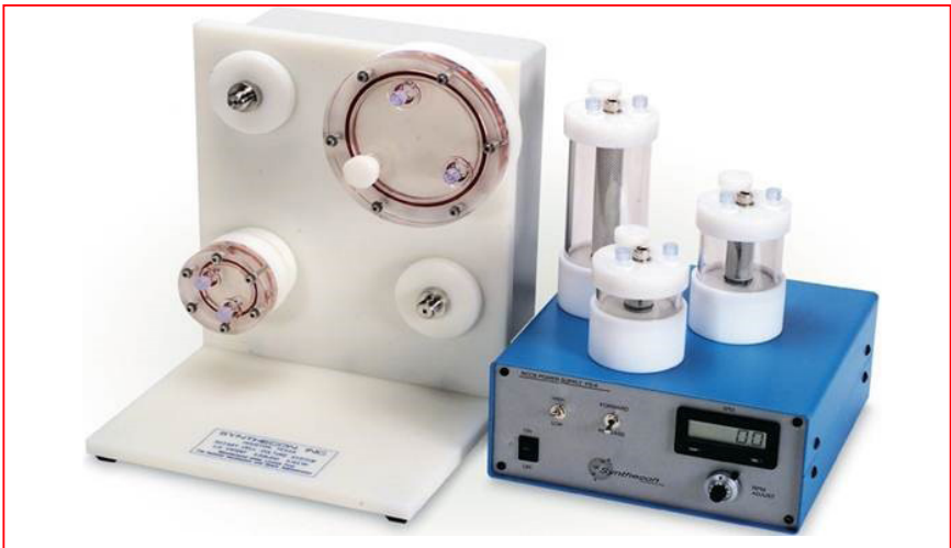
Figure 14: Examples of the rotating-wall vessel bioreactor systems available through Synthecon, Inc., Houston, Texas. Disc-shaped cylindrical vessels on the left are 10-ml and 50-ml high-aspect rotating vessels (HARVs) attached to a four-place rotator base (horizontal-axis rotation). The cylindrical vessels on the right are 55-ml, 110-ml, and 250-ml slow-turning, lateral vessels on top of the power supply positioned as controls (vertical-axis rotation) for the modeled microgravity produced by the HARVs on the left. Source: Synthecon, Inc. ( http://www.synthecon.com/rotary-cell-culture-systems.html ).
