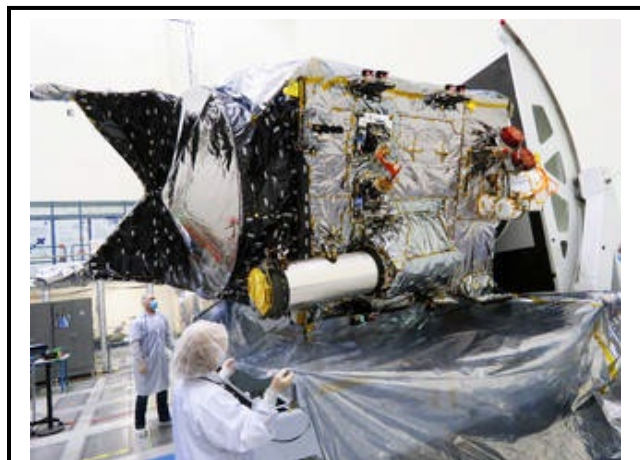
NASA's Deep Space Optical Communications (DSOC) experiment is the agency's first demonstration of optical communications beyond the Earth-Moon system. DSOC is a system that consists of a flight laser transceiver, a ground laser transmitter, and a ground laser receiver. New advanced technologies have been implemented in each of these elements.
