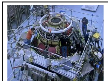
Refurbished Artemis I's Non-Core avionics are being installed on Artemis II Crew Module, shown here.
