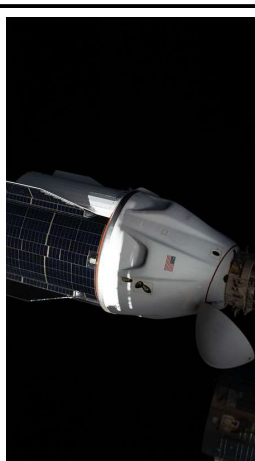
The SpaceX Dragon resupply ship, with its solar panel-covered trunk, is pictured here before undocking from the Harmony module's forward port on the ISS (August 19, 2022).
