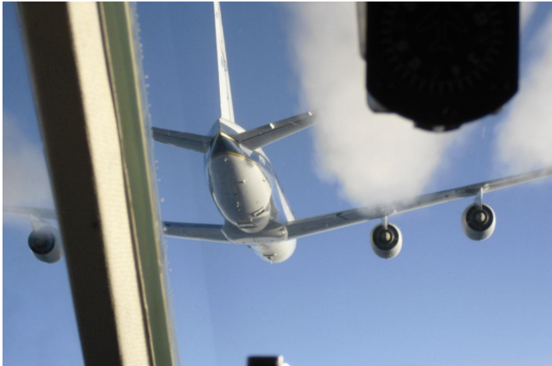
Dryden DC-8 exhaust emissions measured in flight by instrumented Falcon aircraft from Langley
