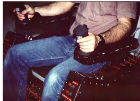
Figure 10.13-2. Deep Rover Control Seat with sliding armrests for vehicle control and two-axis force-sensing control sticks for manipulator control.
