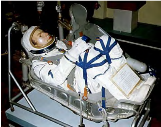
Figure 8.2-8. Soyuz seat. Note the higher degree of flexion in the hips and in the knees compared with the Orion seat in Figure 8.2-6.
