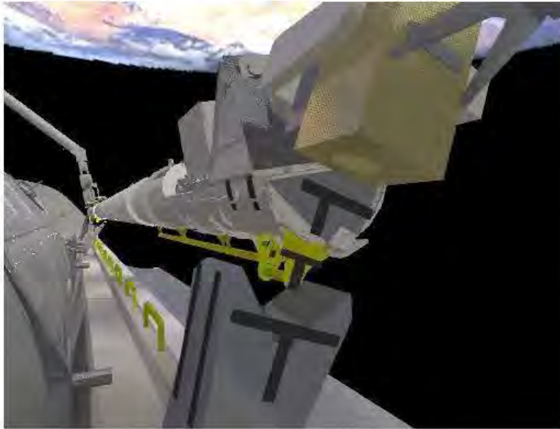
View from Camera C at Dawn +40 minutes, beta angle of 0 degrees, and the OBSS 6 inches away from the berthed position. The lighting is uniform. Image Saturation: 0.00%; Average Luminance: 35 fL. This view is typical for the middle of a day pass for all betas.
