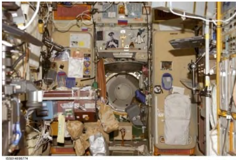
Figure 8.2-5 ISS Russian Service Module with co-located dining table (left), treadmill (bottom), crew sleep quarters (left and right), and toilet (beyond treadmill).
