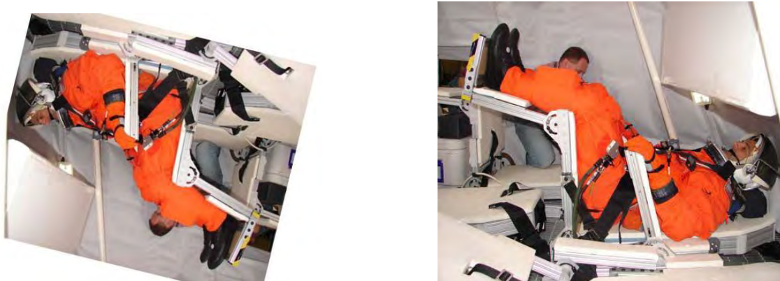
Figure 8.2-6. The image on the left is the approximate position of Orion seat in Stable 2. The image on the right is the Orion seat configuration in a nominal position.
