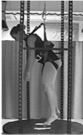
Figure 8.2-7. OSHA-approved full body harness with D-ring attachment point in the mid-back, as studied by NIOSH (reproduced from Turner et al, 2008).
