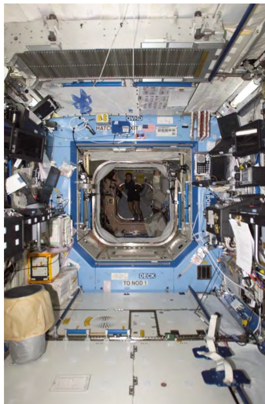
Figure 7.7-1 View of an optimal translation path with minimal rack front stowage from the ISS US Lab.
