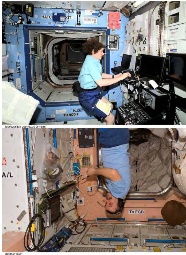
Figure 8.3-6 Endcone paint and labels in the ISS modules Destiny (left) and Unity (right). Top: Astronaut Susan J. Helms, Expedition Two flight engineer, works at a laptop computer in the U.S. Laboratory/Destiny module of the ISS (photo no. ISS002-E-5478, 30 March 2001). Bottom: Cosmonaut Mikhail Tyurin, Expedition 14 flight engineer representing Russia’s Federal Space Agency, uses a communication system as he floats in the Unity node of the ISS (photo no. ISS014-E-12521, 21 Jan. 2007).
