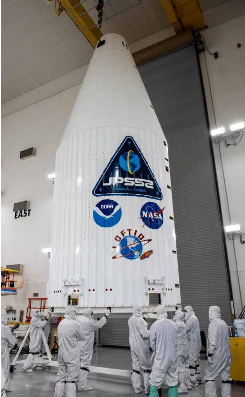
Left: Preparations for Joint Polar Satellite System-2 (JPSS-2) and LOFTID continue with a fit check of the payload fairing inside an Astrotech high bay at Vandenberg Space Force Base. Image Credit: NASA Images
