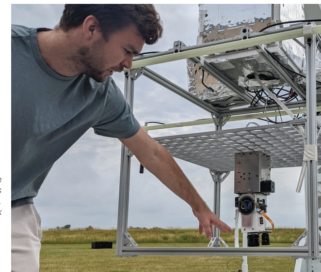
Zachary Gaines, a senior in Cal Poly Pomona’s Bronco Space Lab, points out the camera and sensor used in the team’s Bronco Ember technology to detect and track wildfires. Credits: Aerostar/Anastasia Quanbeck
