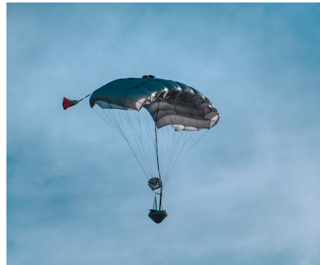
The SpaceWorks RED-4U capsule in flight after being released from a Near Space Corporation high-altitude balloon at 103,000 feet. The parafoil guiding the capsule's descent was developed by Earthly Dynamics and Aerial Delivery Solutions. Credits: SpaceWorks Enterprises, Inc.
