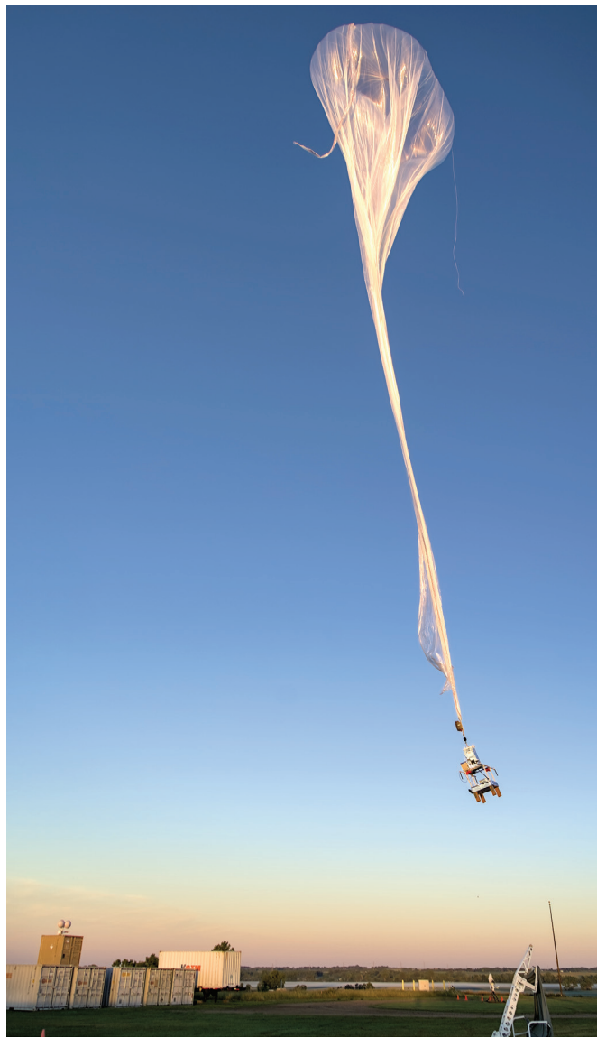
Orion Labs’ Quantum Earth Observatory launches on an Aerostar high-altitude balloon from the company’s facility in Sioux Falls, South Dakota, on July 28, 2022. The observatory hardware is housed in the gondola carried below the balloon. Credits: Orion Labs/Margarita Reyes
