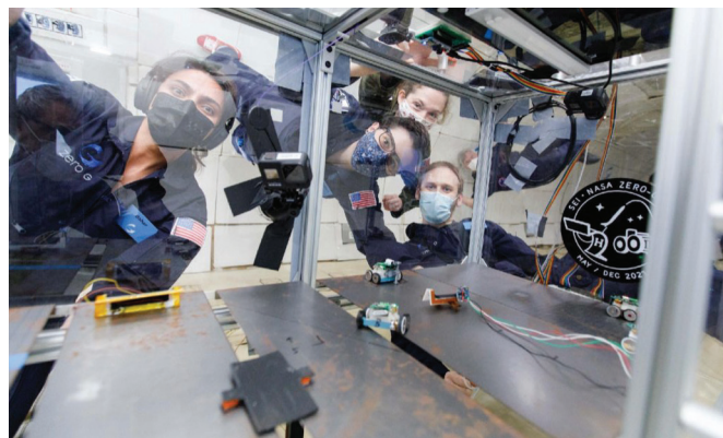
A team of researchers from MIT evaluate the performance of miniature robots for space-based assembly and inspections on a parabolic flight in December 2021. Credits: Zero Gravity Corporation/Steve Boxall
