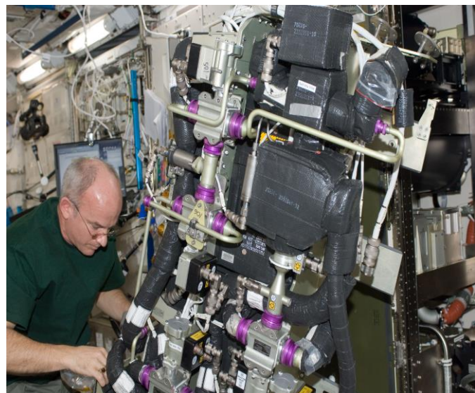
Crewmember performing maintenance on ISS CDRA
