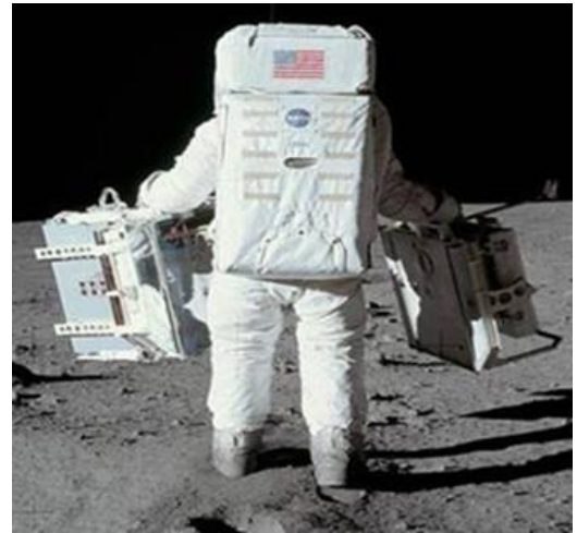
Portable Life Support System PLSS
