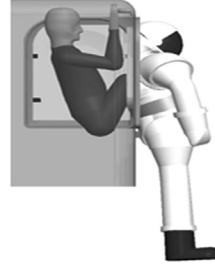
Fig. 2. Suit port egress and ingress procedures (top), prototype (bottom left), and illustration of the egress/ingress method (bottom right).
