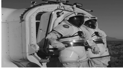
Fig. 2. Suit port egress and ingress procedures (top), prototype (bottom left), and illustration of the egress/ingress method (bottom right).
