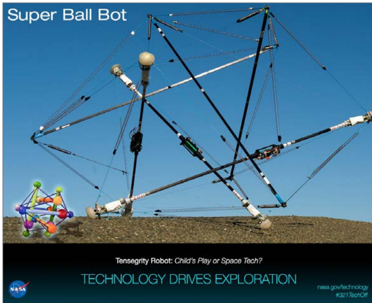
Super Ball Bot is an all-in-one landing and mobility platform based on tensegrity structures, allowing for lower-cost and more reliable planetary missions. (Credit: NASA)
